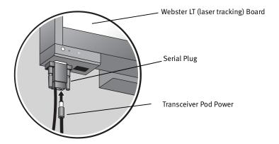
For laser tracking boards, simply plug the barrel connector from the power supply into the serial connector after the serial connector is plugged into the board.
