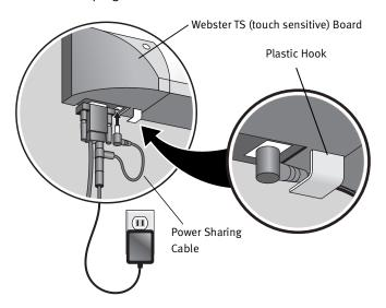
Connect the power supply cable to the barrel socket on the 3 power sharing cable.
