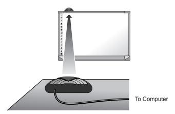
Adjust the position of the computer side pod until you have a green light on both the board and computer side pods. You may also adjust the board side pod. Once in place use the double-sided tape to stick it in place.
