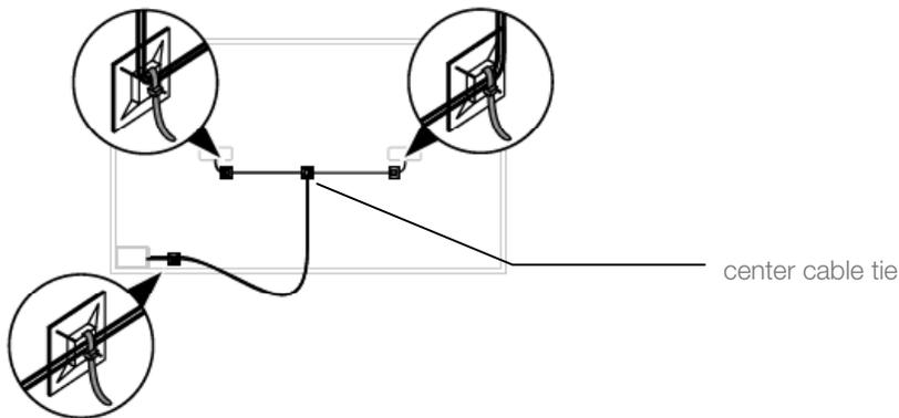
5. Ensure that the driver pack cables are taut between the driver pack and the cable tie.
