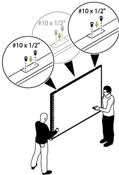
5. Fasten the ēno interactive whiteboard to the upper wall bracket extender using the #10 x 1/2" fasteners provided.
