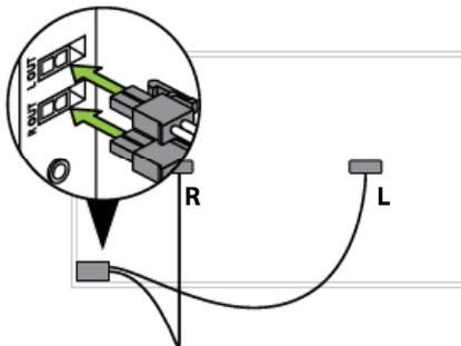
2. Connect the cable from the driver pack on the RIGHT side of the whiteboard to the amplifier connector labeled "L out" for left.
