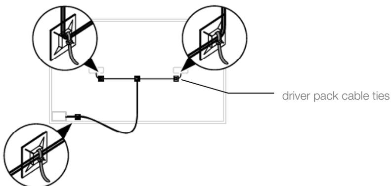
5. Ensure there is about 1/2" service extension between the tie holder and driver pack then tighten the tie wrap.
