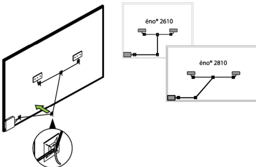
3. Ensure that all cables are taut, then remove self adhesive back from a tie holder.
