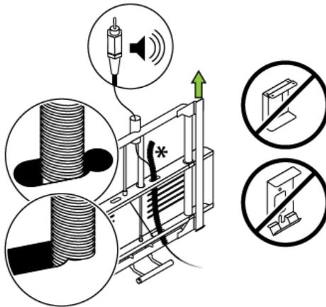
4. Cover cables below the turret base using the split corrugated conduit that is provided with the adjustable height system.
