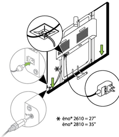
4. Route the cable to the amplifier, making sure that the cable passes between the lift system tubular support structure and the whiteboard, as shown above.
