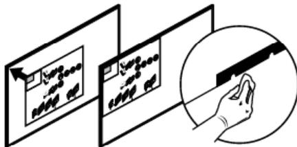
2. Use the illustrations on the template to select the template notches that are appropriate for the type of whiteboard mounting solution in your installation.
