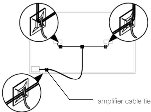
5. Ensure there is about 1/2" service extension between the tie holder and amplifier then tighten the tie wrap.
