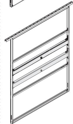
When the cabinet requires two mounting rails, two structural beams must be used accordingly.
