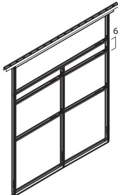
**Posts on either side of a monitor shroud** must extend above the top of the shroud by at least 6".
