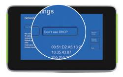
5 Enter an IP address using the keypad.
