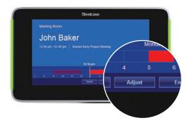
RoomWizard displays the current reservation end time and buttons labeled "+" and "-." Press "+" or "-" to add or remove time from the current reservation.
