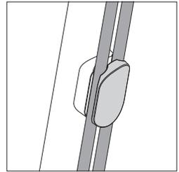
**A cord management system** allows different power and data cords to easily be secured on each leg.
