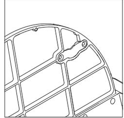
**Seismic locking system** allows for the device to be easily placed on the mobile stand and automatically locks in place.
