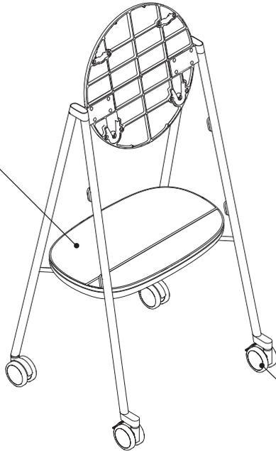
**Mobile stand** includes 360° rotating casters. Front casters are locking and back casters are non-locking.
