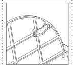
**Seismic locking system** allows for the device to be easily placed on the mobile stand and automatically locks in place.
