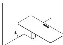
**Power type of no power, plug, or hardwire** is a required selection for wall mounted worksurfaces. No power is available for fixed height worksurfaces. Height adjustable worksurfaces require a selection of either plug or hardwire.
