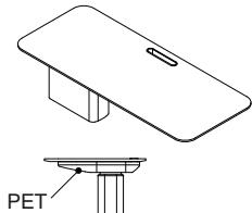
**Worksurfaces** come standard with a PET (polyethylene terephthalate) cover which conceals the worksurface cantilever structure.
