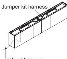
**For an infeed to support multiple foundations**, the infeed must enter and connect to the power block in an end foundation; jumpers connect to adjacent foundations. Power must run in one direction. Infeeds are not able to start in a middle foundation and branch with jumpers in either direction.
