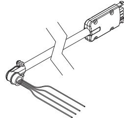
**The hardwire infeed harness** is connected by an electrician to a building junction box, the opposite end of the infeed has a modular connector which plugs into the foundation power block.
