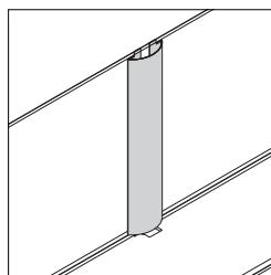
**Monitor mounting kit** includes cable cover, which conceals monitor cables routed into the foundation. Cable cover attaches to the inside of the tower and is fabric wrapped to match the shrouds.
