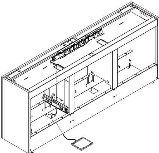
**For applications with foundations,** the permanent power cord is routed through the column, under the foundation, and up to the foundation power block.
