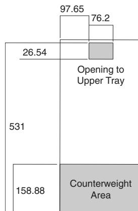
**Access holes in each end of the foundation** allow for jumper harnesses to connect power to adjacent foundations.
