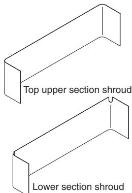
**Tower shrouds for the top upper section of a tower** differ from shrouds in the lower sections, which have a notch for tower shelf frames.
