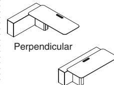
**Personal worksurfaces** can be perpendicular or parallel when planned with foundations or in wall-mount applications.
