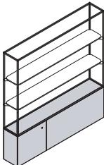
**Towers** attach to foundations to provide space division, shelf storage, and privacy with optional tower shrouds. They must match the width of the foundation and are specified as an option to Mackinac settings.
