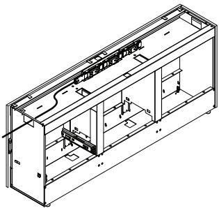
**Building power** may enter the foundation from the end access holes when foundations are perpendicular to a wall and when building power is located in the wall. However, the location of the building wall power junction box must align with access hole.
