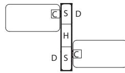
**Configurations which require the HD counterweight package (H)** consist of 30 plates. 15 plates are divided evenly between each section with the remaining 15 placed in the location indicated by H in the Application Guidelines and Assembly Directions.
