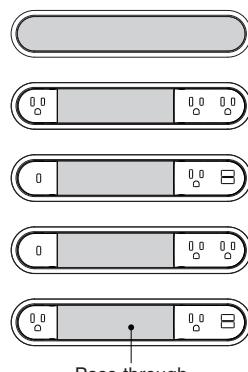
**Surface power** is available with no power (CC grommet only), standard power outlets, USB-A, and USB-C power combinations.
