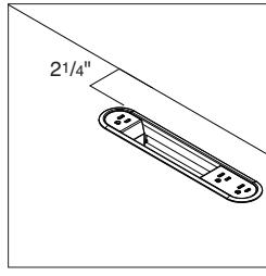
**Personal surface power** is centered along the back edge of the worksurface, 0" from the back edge.
