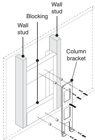
**Wall-mounted worksurfaces** can attach to drywall with either metal or wood studs and require wall blocking.
