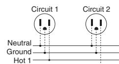
**Mackinac** utilizes a 2-circuit power distribution system with 3 15-amp duplex receptacles supplied with the starter kit and jumper kit.
