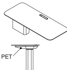
**Worksurfaces** come standard with a PET (polyethylene terephthalate) cover which conceals the worksurface cantilever structure.
