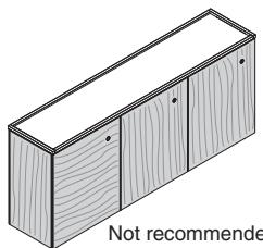
**Opposing grain direction from the foundation** can be specified for individual side skins and drawer fronts; however, it is recommended that all skins within the side match the same direction. If grain direction is mixed on one side, polarization will cause the veneer skins to appear a different color or shade.
