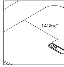
**Collaborative surface power** is centered front to back on the worksurface and 0" from the back edge.
