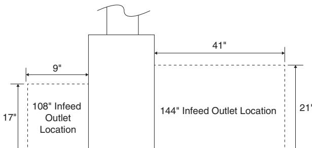
**For wall outlet location planning,** cord lengths will determine the distance from the column to the outlet.
