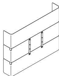
*Tip:* When using the monitor shroud, a worksurface cannot be placed on that side of foundation.
