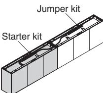
**Jumper kits** provide power to multiple foundations when ganged together replacing the need for multiple starter kits.
