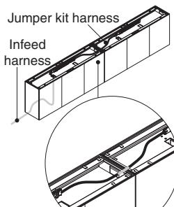
**Infeed harnesses** routes from the building power connection point, underneath the foundation, through access holes up to the foundation top tray and power block.
