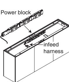
**Foundation power starter kit** is ordered separately for applications with foundations. Two-circuit starter kit includes power infeed harness and foundation power block with 3 15-amp duplex receptacles (6 power outlets).
