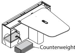
**Foundation counterweights** are required for some configurations, due to the varying weight of the cantilevered worksurface. Some configurations require a standard counterweight package, whereas others require a heavy duty (HD) counterweight package.
