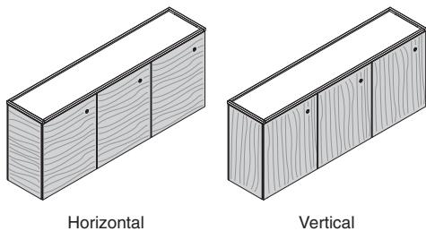
**Wood veneer grain direction** can be specified as either horizontal or vertical for the foundation. End skins will always follow the selection of the foundation grain direction.
