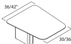
**Collaborative worksurface width** tapers 6" from the back to front edge from 36"W to 30"W and 42"W to 36"W.
