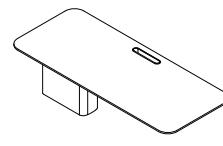
**Permanent power** is not user accessible, as the PET understructure needs to be removed by an installer.
