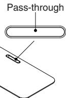
**Personal worksurfaces** are standard with surface power. The CC grommet features a cord pass through to permanent power connections below the worksurface. Surface power comes standard even when the no power or no surface power options are selected.
