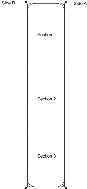
**Mackinac foundations** are split by Side A and B, and Sections 1, 2, and 3. Each section is allowed a drawer, column, or skin. Only one drawer is allowed per foundation section. Only one column is allowed per side. Sides A and B must remain consistent throughout planning.
