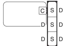
**Configurations which require a standard counterweight package(s)** consists of 15 individual plates. The 15 plates are divided evenly between each foundation section. The plates fit in the foundation cavity below drawers.
