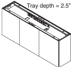
**Ample space within the top channel of the foundation** allows for power infeed harnesses, power and data cables, and power jumpers. Top skin lifts off for access to outlets and connections.
