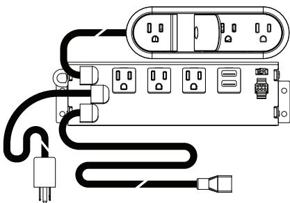
**Power box** is cored with a three prong grounded plug.
