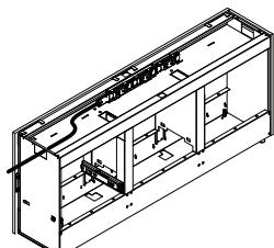
**Harnesses** may route into the end of the foundation if the end skin is removed.
