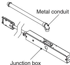
**New York City electrical code** requires hardwiring to building power within a junction box. New York power option includes a junction box, metal conduit, and hardware infeed and foundation power block.
