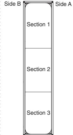
**For planning purposes** foundations are divided into three sections with a designated Side A and Side B. Worksurface columns, drawers, and skins can be positioned in these sections.
