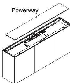
**With powerway on foundation top skin option** must be selected to allow monitor cords to pass through the top skin and plug into the foundation power.
