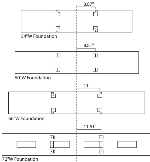
**Location of ingress holes in foundation** is measured from the centerline of the foundation to centerline of the hole.
