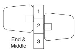
**For dual-sided applications**, they can be placed across from each other, or yin yang, or they can be placed on the end on one side and middle on the other.
