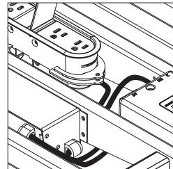
**Height-adjustable worksurface control boxes** require permanent power. The permanent power box includes a cord to connect power to the height-adjustable control box.
