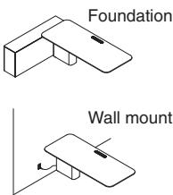
**Worksurfaces** are cantilevered from the column which attaches to the foundation.
