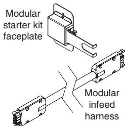
**The modular infeed** includes a wall-mounted modular faceplate that hard-wires directly to the building's power. The infeed has modular connectors on both ends. One end plugs into the faceplate and the opposing end is plugs into the foundation power block. Modular infeeds are only available in 72" L.
