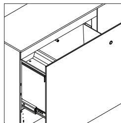
**All drawers** come standard with one file rail, and 0.833 linear feet of filing capabilities. Only front to back filing is accommodated. Legal filing is capable in 60"W foundation drawers and larger. If the personal drawer accessory package is specified, the file rail can not be used.
