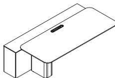
**Personal parallel worksurfaces** can never be longer than the foundation, however, 48"W personal work surface can never be placed parallel.
