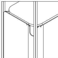
**Tower shrouds in the upper section** are not interchangeable with lower section shrouds, as these shrouds include a cut out for shelf supports.
