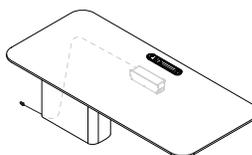
**For wall-mounted applications,** the permanent power cord is routed through the column and exits to plug into a wall or floor box outlet.
