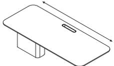
**Personal worksurfaces** are available in modular and parametric sizes with the exception of Corian solid surface. Collaborative worksurfaces are available in modular sizes only.
