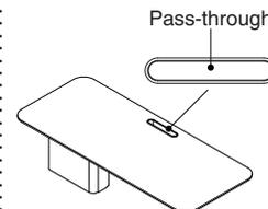
**Personal worksurfaces** are standard with surface power. The CC grommet features a cord pass through to permanent power connections below the work surface. Surface power comes standard even when the no power or no surface power options are selected.
