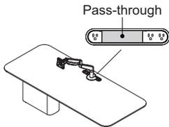
**CF Series monitor arms (listed below) with C-clamp option** can mount through the CC grommets of personal worksurfaces.
