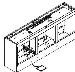
**Infeed harnesses** routes from the building power connection point, underneath the foundation, through access holes up to the foundation top tray and power block.
