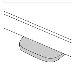
**Simple touch controller** comes standard with height-adjustable worksurfaces and easily adjusts height of work surface at a rate of 1 1/2" per second, by lifting or pressing down on the controller. The controller is mounted on the user side, in line with the column.
