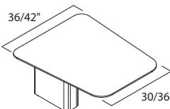
**Collaborative worksurface width** tapers 6" from the back to front edge from 36"W to 30"W and 42"W to 36"W.
