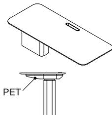
**Worksurfaces** come standard with a PET (polyethylene terephthalate) cover which conceals the work surface cantilever structure.
