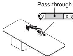
**CF Series monitor arms (listed below) with C-clamp option** can mount through the CC grommets of personal worksurfaces.
