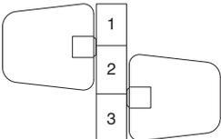
**Collaborative worksurfaces** are non-handed and are allowed to be placed in Sections 1, 2, or 3 when planned with foundations.
