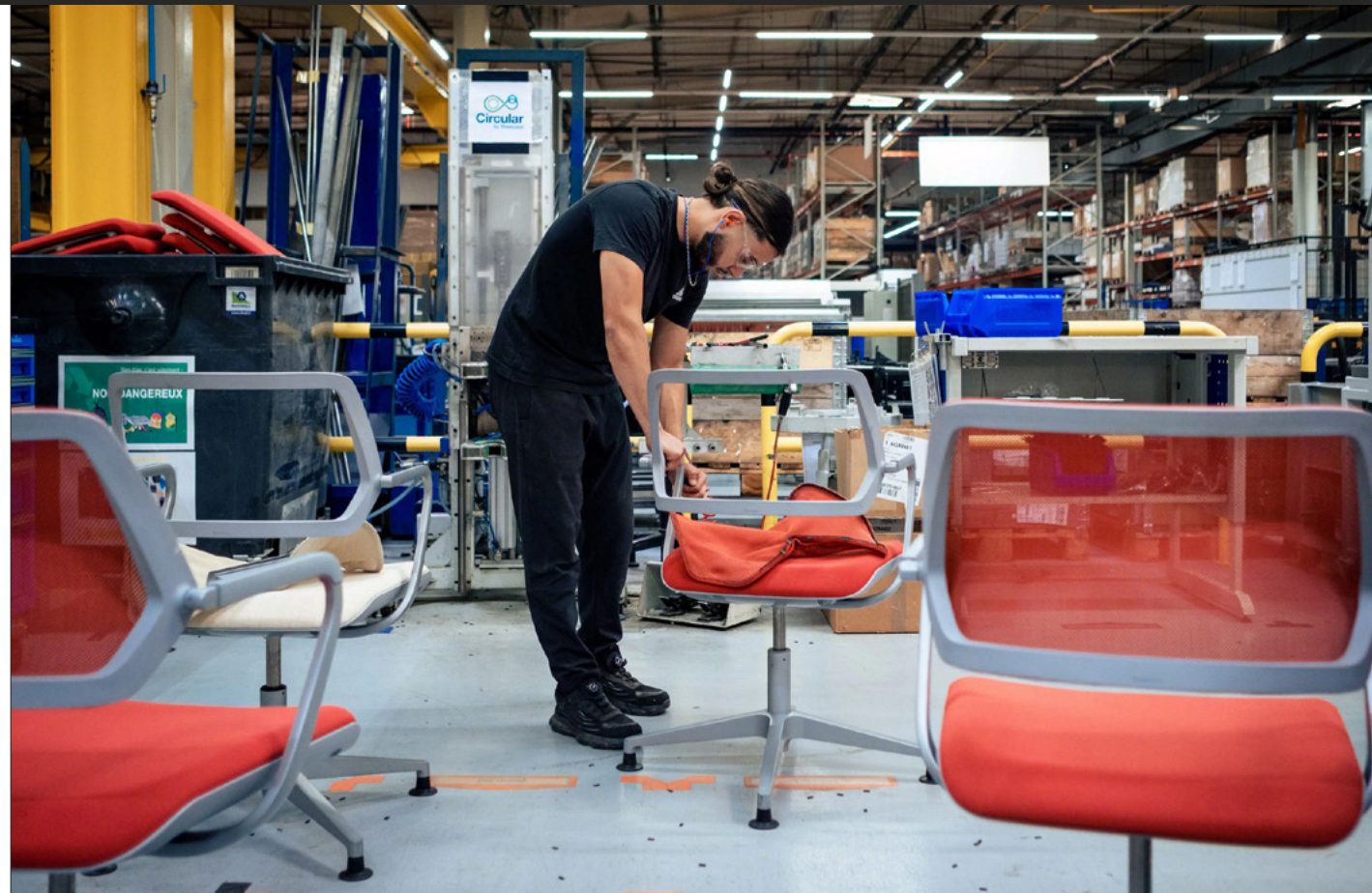
Chair components being replaced during Circular by Steelcase: Remade process, Sarrebourg, France
