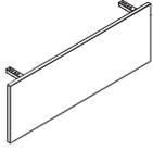
*Tip: Full width modesty panels cannot be used on desks with integrated rail. To use with the integrated rail, the modesty panel must be undersized by a minimum of 20" (rectangular and tapered) or 19" (90°) and 16" (120°), and inset from the edge of the worksurface.*
