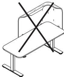
**Flex privacy wrap (FLXDWR)** is not allowed on 23"D worksurfaces or 24"D bow front worksurfaces.
