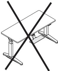
**Keyboard assemblies** are not allowed on rectangle or tapered 24"D or smaller and smaller than 46"W height-adjustable desks. They do not meet minimum safety requirements.
