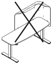
**When attaching 90° desk mount privacy wrap (**FLXDWR**) to 5" radius corners or organic bow front worksurfaces, a worksurface overhang is not allowed on the same side the wrap is mounting.**
