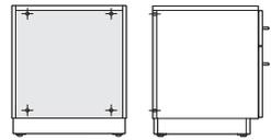
**Base cabinets** must always be fastened to a wall. Attachment hardware is included with cabinets.
