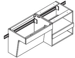
**Printer cabinets** attach to a rail system utilizing a bracket connection. The rail aids in alignment to adjacent cabinets. The rail must be ordered separate from the cabinet.
