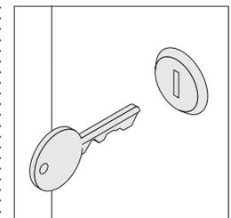
**Locks** are optional and only available with master keying. Locks are field installed and must be specified separately.
