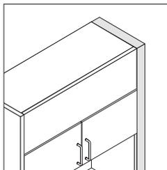
**Fillers** close the gap between the side of a cabinet and a structural wall. Ceiling fillers close the gap between upper microwave cabinets and the ceiling.
