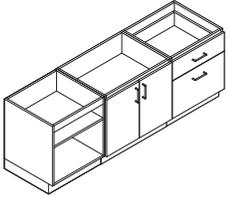
**Bolts** are used to align adjacent cabinets in a multi-unit configuration. The bolts can be removed and reinstalled if a different multi-unit configuration is desired.
