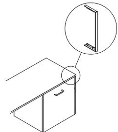
**Wall-suspended base cabinets and upper cabinets** can utilize the wall fillers to enclose the gap between a cabinet and a wall on the front, top, and bottom.
