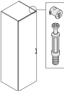
**Cam-lock assembly hardware** is used.
