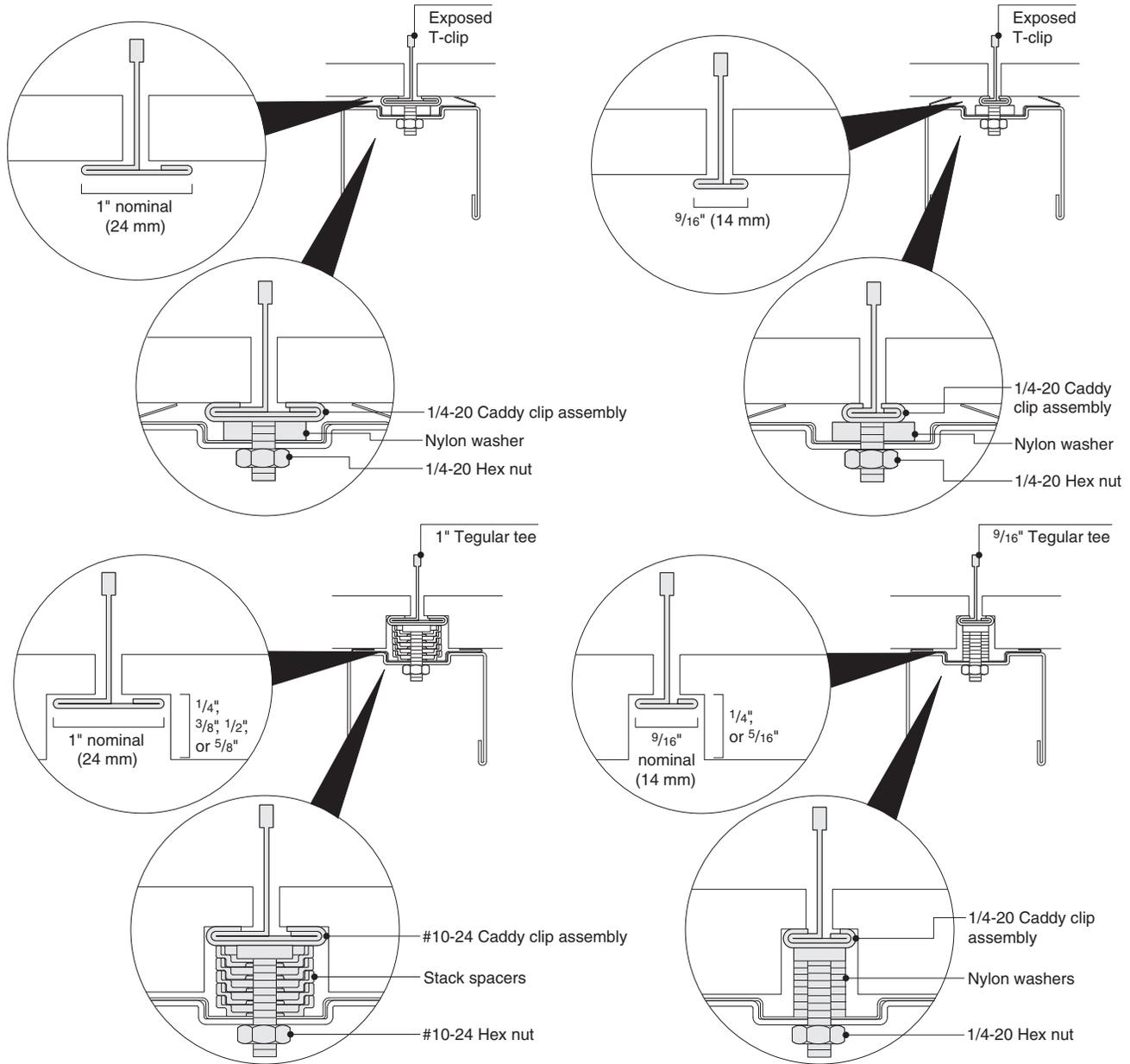
**Bolt Slot Grids Ceiling Fastener Kits**
