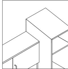
**Upper cabinets** specified with a sloped fascia top condition and installed next to a wardrobe or tall storage cabinet of a different depth will result in a step down. Doors will align between upper cabinet and wardrobe or tall storage. Cover panels will be required in between the wardrobe or tall storage cabinet and upper cabinet.
