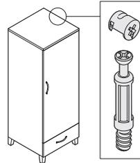
**Cam-lock assembly hardware** is used.
