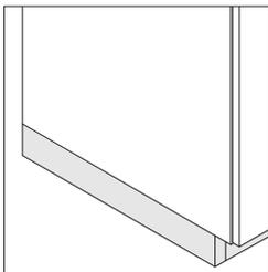
**Base trim** must be added to floor-extended printer cabinets prior to application of cove molding. Base trim is always black. Base trim must be ordered separately. ▶ See page 172 for base trim.
