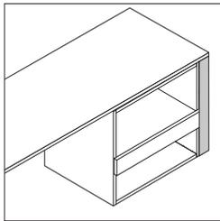
**Fillers** close the gap between the side of a cabinet and a structural wall. ▶ See page 144 for fillers.
