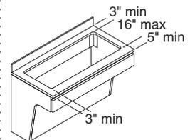
**Maximum sink cutout size** is 16" front to back. Minimum cutout requirements are 5" from front edge and 3" from back and side edges.
