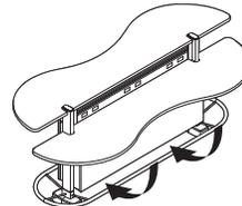
**Airflow** is supported with openings above and below technology stretcher for proper circulation.
