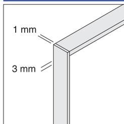
**Edges on cabinets** are matching 1 mm plastic edge banding. Drawer and door edges are matching 3 mm plastic edge banding.
