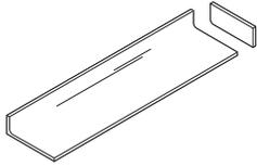
**Solid surface worksurface**, ordered separately, has an integrated backsplash. A solid surface sidesplash is also available in two depths and must be ordered separately.
