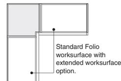
**Corner cabinets** support worksurfaces in a corner application. Field cutting of work surface may be required to achieve architectural fit.
