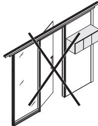
**Hang-on components** should not be mounted in a wall with a door frame (reversible or sliding).
