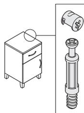
**Cam-lock assembly hardware** is used.
