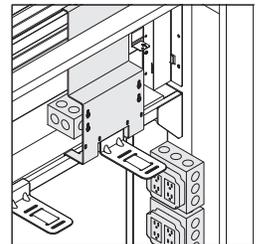
**Junction box mounting locations** are standard. Eight boxes fit into the 72"W and 84"W bases. Twelve boxes fit into 96"W and 108"W bases. Junction boxes are field installed and provided by the electrical contractor.
