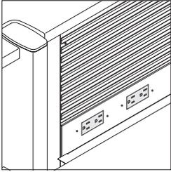
**Receptacle openings** are standard on the lower side of the unit. 72"W units have four openings. 84"W and 96"W and 108"W units have six openings. Receptacles are provided by the electrical contractor.
