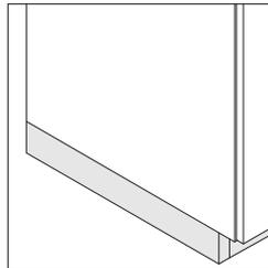
**Base trim** must be added to floor-extended sink base cabinets prior to application of cove molding. Base trim is always black. Base trim must be ordered separately.
