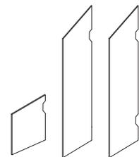
**Depending on the application chosen**, cover panels will either include no cutouts, one top cutout, one bottom cutout, or two cutouts (top and bottom). The cutout provides a space for the continuous rail when in the middle of a run of cabinetry. Refer to SmartTools.
