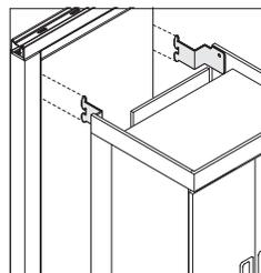
**V.I.A. hang-on bracket option** must be used when mounting to V.I.A. on module. Brackets include one left- and one right-hand bracket.
