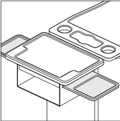
**Supplemental sliding surfaces** are available as an option to provide extra surface space on both sides. This option reduces the height of the open cubby from 6.4" to 4.05".
