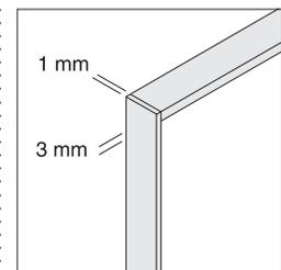
**Edge**, on cabinets are matching 1 mm plastic edge banding. Door edges are matching 3 mm plastic edge banding.
