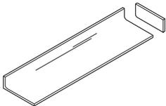
**Solid surface work surface**, ordered separately, has an integrated backsplash. A solid surface sidesplash in two depths is also available and must be ordered separately.
