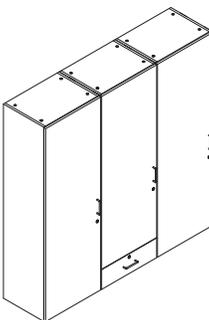
**Bolts** are used to align adjacent cabinets in a multi-unit configuration. The bolts can be removed and reinstalled if a different multi-unit configuration is desired.
