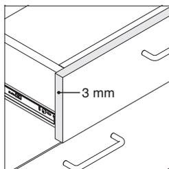
**Edges of drawer fronts** are complimenting 3 mm edge band for increased durability in a high touch point space. Contrasting edge band is not offered.
