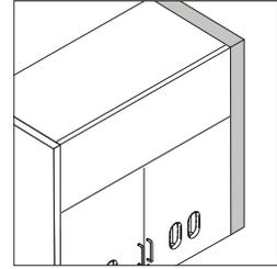
**Fillers** close the gap between the side of a cabinet and a structural wall. Ceiling fillers close the gap between upper cabinets and the ceiling.
