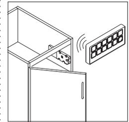
**Electronic locks** are optional and field installed. Lock receivers can be installed on drawers and doors and are wirelessly controlled by a transmitter.
