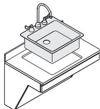
**Sink** must be independently purchased and field installed. Sink cutout must be cut in field.
