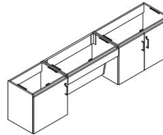
**Bolts** are used to align adjacent cabinets in a multi-unit configuration. The bolts can be removed and reinstalled if a different multi-unit configuration is desired.
