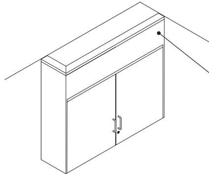
**Vertical fascia** includes a track system to fit into a grid system or direct to dry wall.
