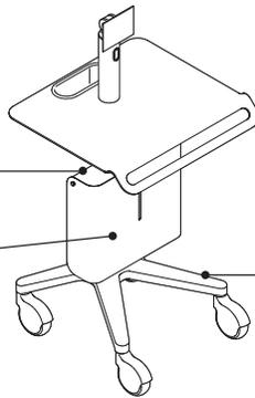
**Monitor mount** is standard on 25"x24" top surface. 75 and 100MM VESA mount allows for 20 pound capacity. VESA mount is adjust-able for various angles on the vertical axis and accommodates cables. Monitor mount adds 13 1/2" to overall height.
