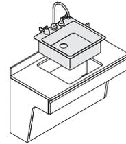
**Sink** must be independently purchased and field installed. Sink cutout must be cut in field. For clinical sink application guidelines, see *Folio Technical Cut Sheet*, available at [village.steelcase.com](http://village.steelcase.com).
