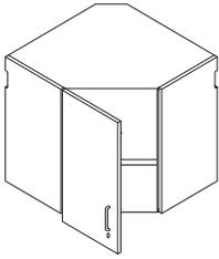
**Cabinets** are hinged on the left or right side. A left-hand unit has the hinge on the left side of the door. A right-hand unit has the hinge on the right side of the door.
