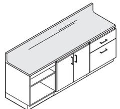
**Worksurface** is available to connect to one cabinet or to span multiple cabinets. It fastens to the top of cabinet with brackets and is field-installed. Brackets are included as standard with base cabinets.
