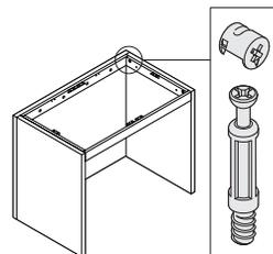
**Cam-lock assembly hardware** is used.
