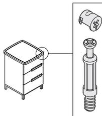
**Cam-lock assembly hardware** is used.
