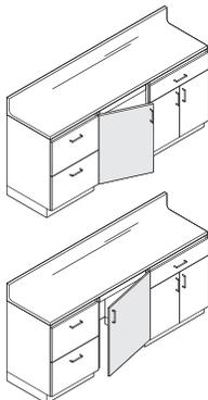
**Desk frames with the single-door option** are hinged on the left or right side. A left-hand unit has the hinge on the left side of the door. A right-hand unit has the hinge on the right side of the door.
