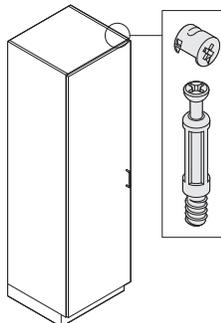
**Cam-lock assembly hardware** is used.
