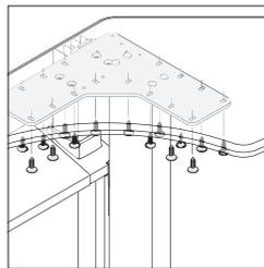
**Worksurface** is secured by use of the surface mounting plate which is standard with the base.
