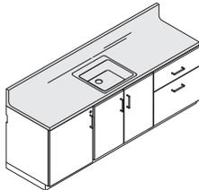
**Worksurface** will span entire length of run of cabinets, up to 138"W for solid surface worksurfaces and up to 120"W for High-Pressure Laminate worksurfaces.
