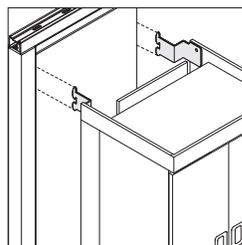
**V.I.A. hang-on bracket option** must be used when mounting to V.I.A. on module. Brackets include one left- and one right-hand bracket.
