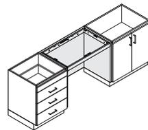
**Base or sink cabinets, or structural wall**, must be attached to one or both sides of desk frame.
