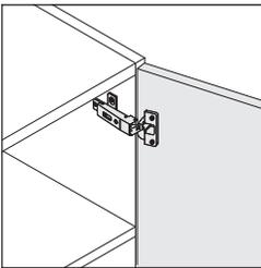
**Euro hinge** is standard on cabinet door and allows the door to open a full 110°.
