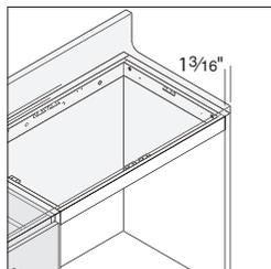
**Extended worksurface** option is available and adds 13/16" length to the worksurface for attachment to one support end panel. Support end panel must be ordered separately.
