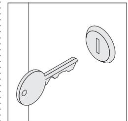
**Lock** is optional and factory- or field-installed to secure the doors. Factory-installed locks are available keyed random only. Optional field-installed locks are available with consecutive, specific, or random keying options. Master-keyed locks are also available. Field-installed lock cylinders must be specified separately.
