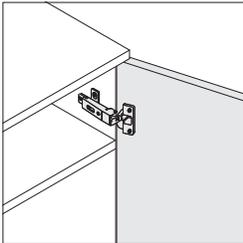
**Euro hinge** is standard on cabinet doors and allows the door to open a full 110° for easy access.
