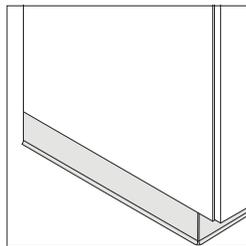
**Cove molding** must be field installed onto the garage cabinet base to complete an installation and is supplied locally. See *Convey Technical Cut Sheet*, available at [village.steelcase.com](http://village.steelcase.com).
