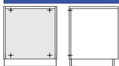
**Corner cabinets** must always be fastened to a wall. Attachment hardware is included with cabinets.
