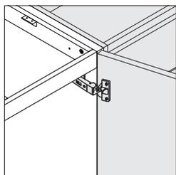
**Euro hinge** is standard on units with doors and allows the door to open a full 110°.
