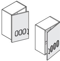
**Single-door cabinets** are hinged on the left or right side. A left-hand unit has the hinge on the left side of the door. A right-hand unit has the hinge on the right side of the door.
