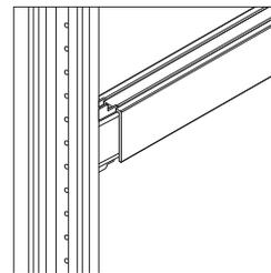
**Convey rails** attach to the structural beam by screwing through the skins. The V.I.A. spacer is required to fill the gap between the skin and the beam. Spacers are not visible once the skin is in place. Spacers span the width of the structural beam.
