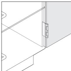
**Five-knuckle hinge** is optional on units with doors and allows the door to open 270° or 180° if connected to adjacent cabinet.
