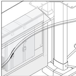
**Top cap and tile** can be removed for easy accessibility to technology and CPUs.
