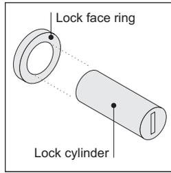
**Locks** consist of a factory- or field-installed lock cylinder and a factory-installed lock face ring.
