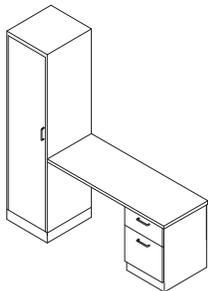
**Worksurfaces** can attach to the top of one base cabinet or can span entire length of run of cabinets, up to 138"W for solid surface worksurfaces and up to 120"W for High-Pressure Laminate worksurfaces.
