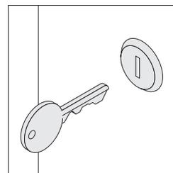
**Locks** are optional and only available with master keying. Locks are field installed and must be specified separately. ▶ *Lock and Keying*, page 398
