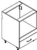
**When adding a drawer to the printer cabinet,** cabinets 24"W or less will include a single drawer. Cabinets 25"W or wider default to two drawers, side by side.
