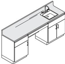
**Worksurface** is available to connect to one cabinet or to span multiple cabinets. It fastens to the top of cabinet with brackets and is field-installed. Brackets are included as standard with base cabinets.
