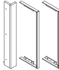
**Wall fillers** enclose the space between a cabinet and a wall on the front, top, and bottom.
