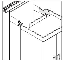
**V.I.A. hang-on bracket option** must be used when mounting to V.I.A. on module. Brackets include one left- and one right-hand bracket.
