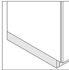
**Base trim** must be added under base cabinet prior to application of cove molding. Cove molding is applied over base trim and is generally supplied by general contractor or client and must be coordinated. Base trim is always black.
