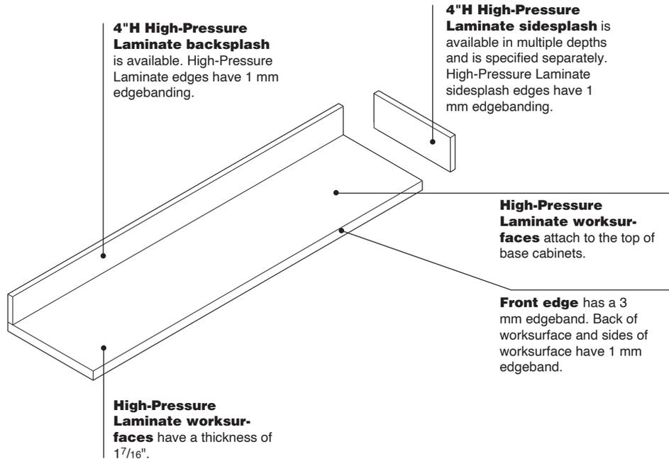
**High-Pressure Laminate worksurfaces** attach to the top of base cabinets.
