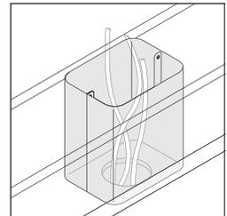
**Base power-in cover** mounts to floor to allow cables to run from the floor into the unit.
