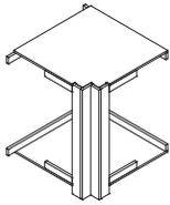
Tip: Fillers close the gap between a cabinet and structural wall. Field cutting of filler may be required to achieve architectural fit.
