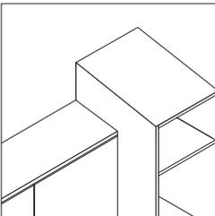
**Storage cabinets** specified with a sloped fascia top condition, and installed next to an upper cabinet of a different depth, will result in a step down. Doors will align between upper cabinet and tall storage cabinets. Cover panels will be required in between the storage cabinet and upper cabinet.
