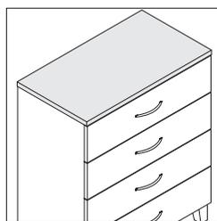
**Solid surface top** is available as an option on cabinets with Low-Pressure Laminate or wood fronts only.
