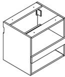
**Printer cabinets without a drawer** will have an open cavity below the pull-out shelf. The open cavity is 6 3/8"H.
