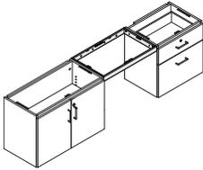
**Base or sink cabinets, or structural wall**, must be attached to one or both sides of desk frame.
