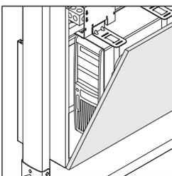
**Tile** can snap open for easy accessibility to technology and CPUs. Straps hold the tile in the open position and can be released to remove tile completely.
