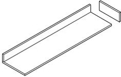
**High-Pressure Laminate work surface**, ordered separately, is available with High-Pressure Laminate. High-Pressure Laminate has a matching 3 mm plastic front edge and 1 mm plastic edge on sides and back. Backsplash is standard with the work surface. High-Pressure Laminate side-splash is also available in two depths and must be ordered separately.
