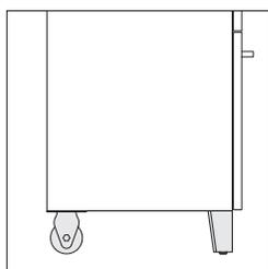
**Rear rollers and front glides** are optional to assist in moving the table. When selecting option for metal or enclosed base, rear rollers are non-directional and are placed adjacent to the rear legs. When selecting option for wood base, rear rollers are non-directional and replace rear legs.
