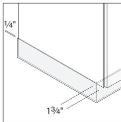
**Cove molding** must be field installed on base to complete installation. The front base of cabinet is recessed 1 3/4". The sides and back are set in 1/4" to allow cove molding to fit flush. Cove molding must be supplied locally.
