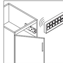
**Electronic locks** are optional and field installed. Lock receivers can be installed on drawers and doors and are wirelessly controlled by a transmitter.
