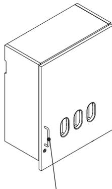
**D pulls** are standard on doors in a nickel finish. Additional finishes and pull options are available.
