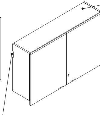
**Notches** must be covered by cover panels or a notch filler for end-of-run conditions.
