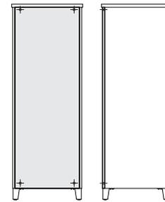
**Wardrobe cabinets** must always be fastened to a wall. Attachment hardware is included with cabinets.
