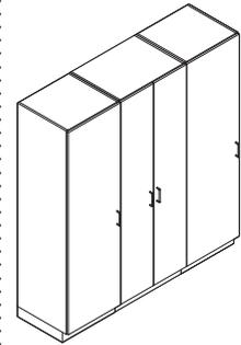
**Bolts** are used to align adjacent cabinets in a multi-unit configuration. The bolts can be removed and reinstalled if a different multi-unit configuration is desired. *Tip: Side of cabinet will be defaced by bolts. Exposed bolt holes will require field fix.*
