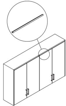
**Upper cabinets, wardrobe cabinets, and tall storage cabinets** utilize the ceiling filler to enclose the gap between the cabinets and the ceiling or bulkhead.
