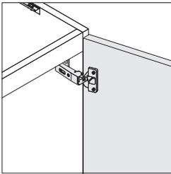
**Euro hinge** is standard on cabinet door and allows the door to open a full 110°.
