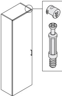
**Cam-lock assembly hardware** is used.
