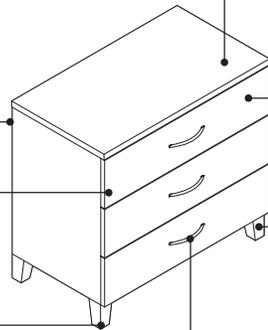
**Drawer fronts** are rigid thermoform or Low-Pressure Laminate.
