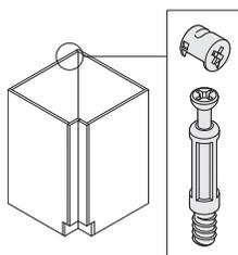
**Cam-lock assembly hardware** is used.
