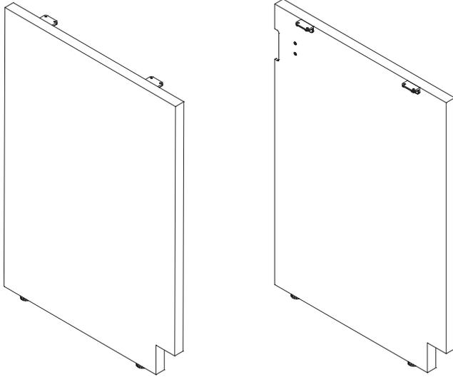
**End panels** can be specified as left hand or right hand. This determines which side of the end panel will be finished, and which will be notched for the rail location.
