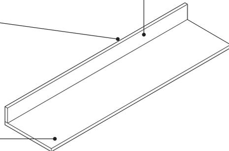
**High-Pressure Laminate worksurface and backsplash** have a particle board core with a High-Pressure Laminate surface.
