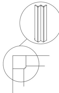
**Floor-extended base cabinets** can utilize the floor-extended corner filler to enclose the gap where the corners meet.
