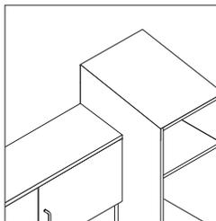
**Microwave upper cabinets,** specified with a sloped fascia top condition and installed next to a wardrobe or tall storage cabinet of a different depth, will result in a step down. Doors will align between microwave cabinet and wardrobe or tall storage. Cover panels will be required in between the wardrobe or tall storage cabinet and upper microwave cabinet.
