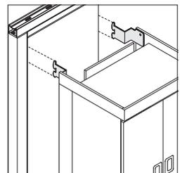
**V.I.A. hang-on bracket option** must be used when mounting to V.I.A. on module. Brackets include four left- and four right-hand brackets.
