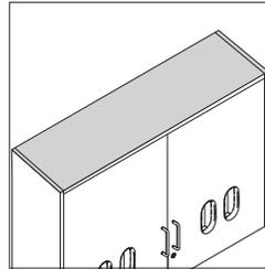
**Sloped fascia, vertical fascia, or flat top-cap cover panels** can be specified as a top condition on the upper cabinets.
