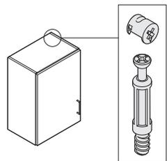
**Cam-lock assembly hardware** is used.
