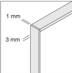
**Edges on cabinets** are matching 1 mm plastic edge banding. Door edges are matching 3 mm plastic edge banding.
