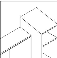
**Wardrobe cabinets** specified with a sloped fascia top condition, and installed next to an upper cabinet of a different depth, will result in a step down. Doors will align between upper cabinet and wardrobe cabinet. Cover panels will be required in between the wardrobe cabinet and upper cabinet.
