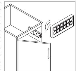
**Electronic locks** are optional and field installed. Lock receivers are installed on drawers and doors and are wirelessly controlled by a transmitter.
