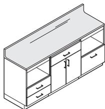
**Work surface** is available to connect to one cabinet or to span multiple cabinets. It fastens to the top of cabinet with brackets and is field-installed. Brackets are included as standard with base cabinets.
