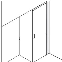
**Fillers** close the gap between the side of a cabinet and a structural wall. Ceiling fillers can also be specified to fill the gap between the top of a wardrobe cabinet and a structural ceiling.
