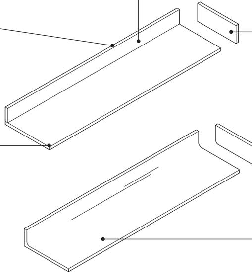
**Sidesplash in High-Pressure Laminate or solid surface** is available in two depths to accommodate various applications. High-Pressure Laminate sidesplash is non-handed. Solid surface sidesplash is available right- or left-handed. Sidesplashes must be ordered separately.
