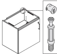
**Cam-lock assembly hardware** is used.
