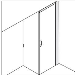
**Fillers** close the gap between the side of a cabinet and a structural wall. Ceiling fillers can also be specified to fill the gap between the top of a tall storage cabinet and a structural ceiling.
