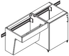
**Base cabinets** attach to a rail system utilizing a bracket connection. The rail aids in alignment to adjacent cabinets. The rail must be ordered separate from the cabinet.
