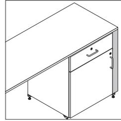
**Fillers** close the gap between the side of a cabinet and a structural wall.
