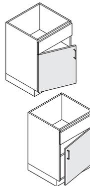
**Single-door cabinets** are hinged on the left or right side. A left-hand unit has the hinge on the left side of the door. A right-hand unit has the hinge on the right side of the door.
