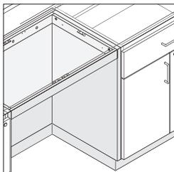
**When desk frame with back panel** is selected, side panels are included. This unit is nominally 31" in height, it is meant to be used in conjunction with the 35"H base cabinets or end panels. It is not meant to be freestanding, nor to be used on the end of a run with additional support. Side and back panels extend to the top of the base of the adjacent cabinet to allow for easy installation of the cove molding.
