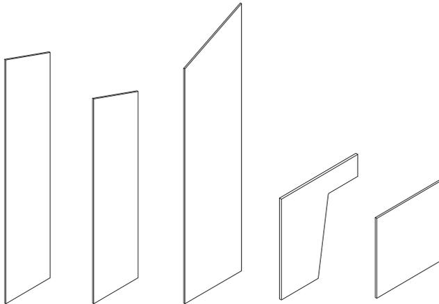
**Cover panels** attach directly to the side of casework.
