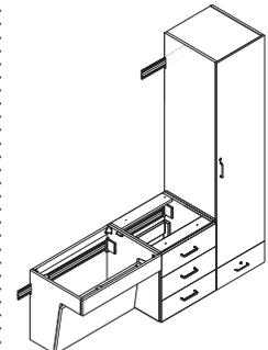
**Cabinets** attach to a rail system utilizing a bracket connection. The rail aids in alignment to adjacent cabinets. The rail must be ordered separate from the cabinet.
