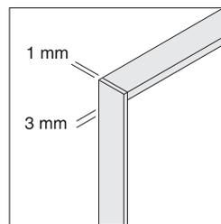
**Edge**, on cabinets are matching 1 mm plastic edge banding. Door edges are matching 3 mm plastic edge banding.
