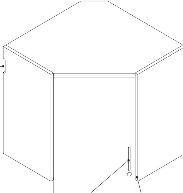
**All edges** are finished from the factory with matching plastic edge banding.
