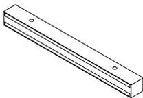
*Tip: Attaching rail to unit will add to overall footprint of cart. Rail is approximately 12<sup>1</sup>/<sub>2</sub>" in length and 1<sup>3</sup>/<sub>16</sub>" in depth and height.*
