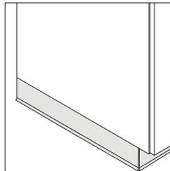
**Cove molding** must be field installed on base trim to complete an installation and is supplied locally. The base trim on the cabinet is inset. See *Convey Technical Cut Sheet*, available at [village.steelcase.com](http://village.steelcase.com).
