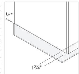
**Cove molding** must be field installed on base to complete installation. The front base of cabinet is recessed 1 3/4". The sides and back are set in 1/4" to allow cove molding to fit flush. Cove molding must be supplied locally. Sink cabinets with angled fronts do not extend fully to the floor and do not require cove molding.
