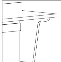
**Exposed rail under the worksurface** can be concealed using a rail cover. ▶ See page 168 for accessories.
