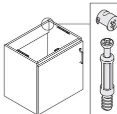
**Cam-lock assembly hardware** is used.
