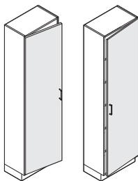
**Single-door cabinets** are hinged on the left or right side. A left-hand unit has the hinge on the left side of the door. A right-hand unit has the hinge on the right side of the door.
