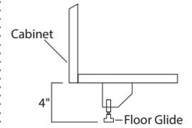
**Floor extended cabinetry** includes floor glides at all four corners allowing for 2" of adjustment on uneven floors.
