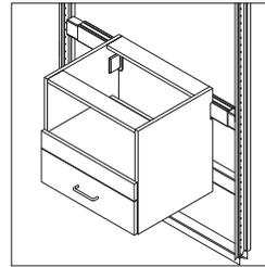
**Base cabinets** cannot be planned at 28 1/2" surface height as there is not enough room to support the structural beams needed at the bottom and top of the case.
