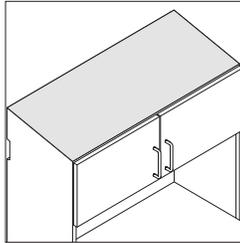
**Sloped fascia, vertical fascia, or flat top-cap cover panels** can be specified as a top condition on the microwave cabinet.
