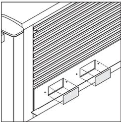
**Receptacle opening fillers** fill in the electrical cutouts when not required and are ordered separately, as a customer service part, 943102877SR.
