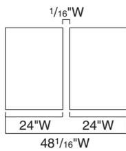
**For appropriate fit and finish a 1/16" gap** is created between adjacent cabinets. For example: Two 24"W side-by-side cabinets will actually be 48 1/16"W.
