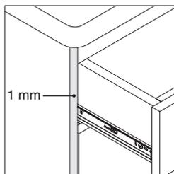
**Edges of cabinet cases** are complimenting 1 mm edge band. Contrasting edge band is not offered.
