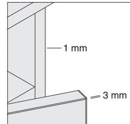
**Edges on cabinet cases** are matching 1 mm plastic trim for Low-Pressure Laminate. Drawer and door edges are matching 3 mm plastic trim for Low-Pressure Laminate. Rigid thermoform drawer and door fronts have the edges wrapped in thermoform foil.
