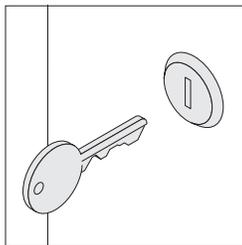
**Lock** is optional and factory- or field-installed to secure the doors. Factory-installed locks are available keyed random only. Optional field-installed locks are available with consecutive, specific, or random keying options. Master-keyed locks are also available. Field-installed lock cylinders must be specified separately.
