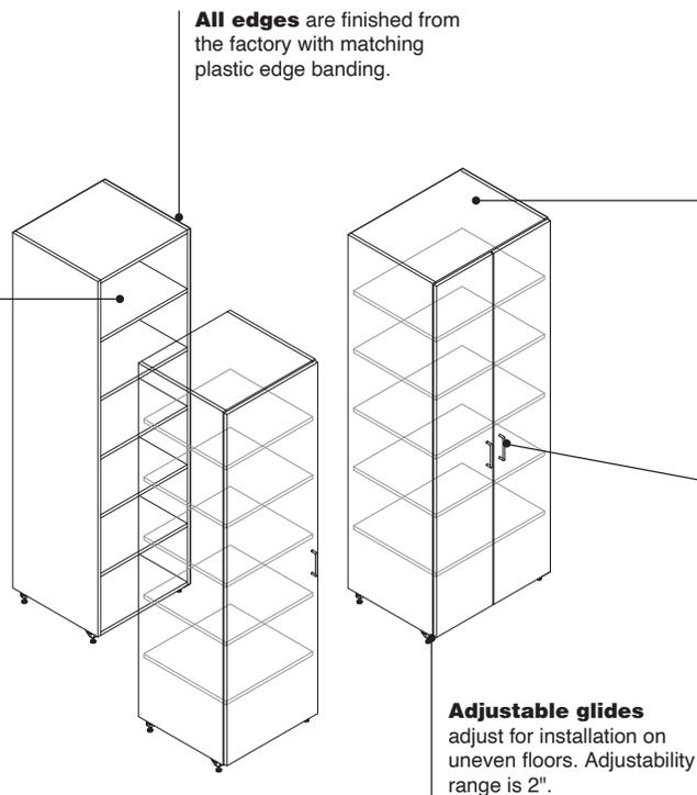
**Base trim** must be added to storage cabinets prior to application of cove molding. Cove molding is required and is to be supplied by others. Base trim is always black. Base trim must be ordered separately.
