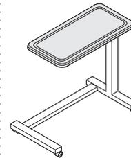
**Spill collector top** includes a trough to collect and prevent liquids from spilling over the edge.
