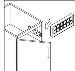
**The transmitter pad** operates within a 15' range. Keypads are user programmable with optional modes of operations for single-use or self-lock.
