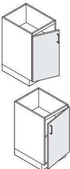
**Single-door cabinets** are hinged on the left or right side. A left-hand unit has the hinge on the left side of the door. A right-hand unit has the hinge on the right side of the door.
