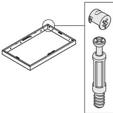
**Cam-lock assembly hardware** is used.
