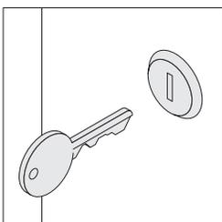
**Lock** is optional and factory- or field-installed to secure the doors or top drawer of the cabinet. Factory-installed locks are available keyed random only. Optional field-installed locks are available with consecutive, specific, or random keying options. Master-keyed locks are also available. Field-installed lock cylinders must be specified separately.
