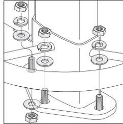
**Floor attachment bolts** are not provided with the unit. The Engineer of Record must specify appropriate attachment hardware. Plate loading information is available at [village.steelcase.com](http://village.steelcase.com) or by contacting 1.800.342.8562. Bolts will secure the leg to the floor and will utilize a leveling system to provide the stability on uneven floors. Template is available to position loading plates to aid installation.
