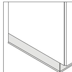
**Cove molding** must be field installed on base trim to complete an installation and is supplied locally. The base trim on the cabinet is inset. See *Convey Technical Cut Sheet*, available at [village.steelcase.com](#).
