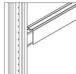
**Convey rails** attach to the structural beam by screwing through the skins. The V.I.A. spacer is required to fill the gap between the skin and the beam. Spacers are not visible once the skin is in place. Spacers span the width of the structural beam. ▶ See page 178 for V.I.A. spacer.
