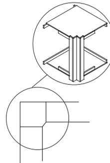
**Upper cabinets and wall-suspended base cabinets** utilize the side corner filler to enclose the space made where the corner meets. This includes the reveal, the top, and bottom of the run.
