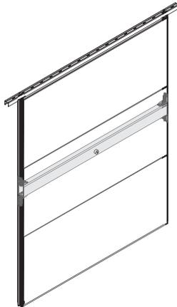
**Reinforcing structural beams (FEBSTR)** must be specified to allow cabinet to attach off module to V.I.A. There is no weight applied to the skin itself.
