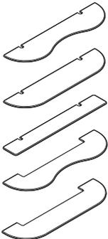
**Worksurfaces** are available in three shapes: interaction, process, and transaction for upper worksurface heights and two shapes: interaction and process for lower worksurface heights.
