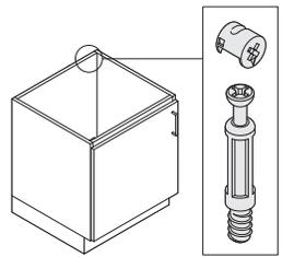
**Cam-lock assembly hardware** is used.
