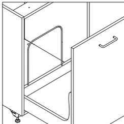
**A removable wire hoop** is included in the pullout drawer to hold customer supplied interior bins in place.
