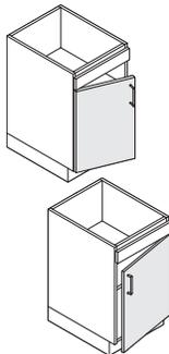
**Single-door cabinets** are hinged on the left or right side. A left-hand unit has the hinge on the left side of the door. A right-hand unit has the hinge on the right side of the door.
