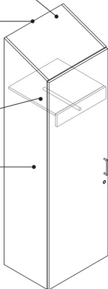
**All edges** are finished from the factory with matching plastic edge banding.
