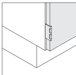
**Five-knuckle hinge** is optional and allows the door to open 270° or 180° if connected to adjacent cabinet.
