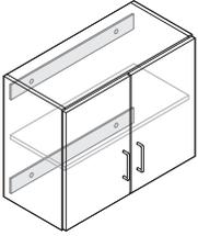
**Cleat systems** must be used when mounting to drywall. Mounting cleats and attachment hardware are included with upper storage cabinets. Check local codes.
