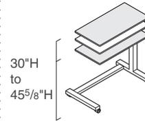
**Adjustable-height C-base** allows the table top height to be positioned in a 30"H–45<sup>5</sup>/<sub>8</sub>"H range (to top of table).
