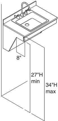
**ADA sink cabinets** meet the guidelines as set forth in the United States Department of Justice 2010 ADA Standards for Accessible Design ([www.ada.gov/2010A-DA-standards](http://www.ada.gov/2010A-DA-standards)). Floor to underside of cabinet clear dimension is 27"H.
