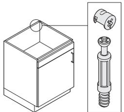
**Cam-lock assembly hardware** is used.
