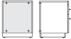
**Base cabinets** must always be fastened to a wall. Attachment hardware is included with cabinets.
