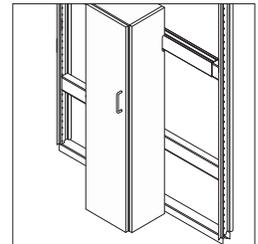
**Base cabinets** cannot be planned at 28 1/2" surface height as there is not enough room to support the structural beams needed at the bottom and top of the case.
