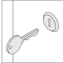
**Lock** is optional and factory- or field-installed on single-door and double-door wardrobe cabinets without drawers. Factory-installed locks are available with consecutive, specific, or random keying options. Master-keyed locks are also available. Field-installed lock cylinders must be specified separately.
