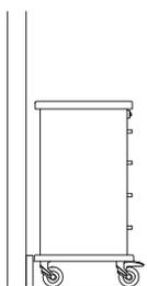
**Cart outer base** protects walls by interacting with walls before the case.
