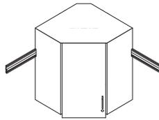
**Upper corner cabinets** attach to a rail system utilizing a bracket connection. The rail aids in alignment to adjacent cabinets. The rail must be ordered separate from the cabinet.
