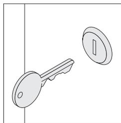
**Lock** is optional and factory- or field-installed to secure the top drawer of the cabinet. Factory-installed locks are available keyed random only. Optional field-installed locks are available with consecutive, specific, or random keying options. Master-keyed locks are also available. Field-installed lock cylinders must be specified separately.
