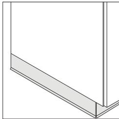
**Cove molding** must be field installed on base trim to complete an installation and is supplied locally. The base trim on the cabinet is inset. See the *Convey Technical Cut Sheet*, available at [village.steelcase.com](http://village.steelcase.com).
