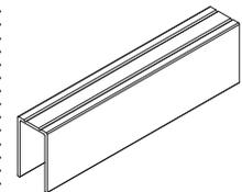
**Convey rails** attach to the structural beam by screwing through the skins. The V.I.A. spacer is required to fill the gap between the skin and the beam. Spacers are not visible once the skin is in place. Spacers span the width of the structural beam. ▶ See page 178 for V.I.A. spacer.
