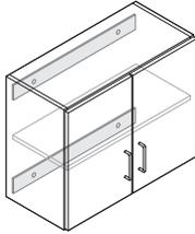
**Cleat systems** must be used when mounting to drywall. Mounting cleats and attachment hardware are included with upper storage cabinets. Check local codes.
