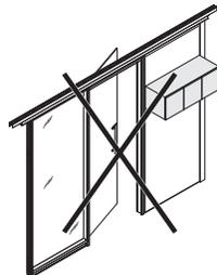
**Cabinets** can be mounted from both faces of a structural beam.
