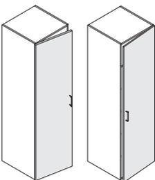
**Single-door cabinets** are hinged on the left or right side. A left-hand unit has the hinge on the left side of the door. A right-hand unit has the hinge on the right side of the door.
