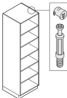
**Cam-lock assembly hardware** is used.
