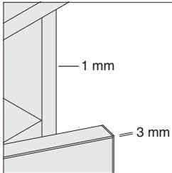
**Edges on cabinet cases** are matching 1 mm plastic trim for Low-Pressure Laminate. Drawer and door edges are matching 3 mm plastic trim for Low-Pressure Laminate. Rigid thermoform drawer and door fronts have the edges wrapped in thermoform foil.
