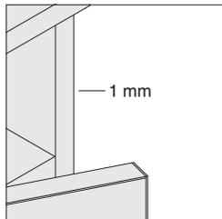
**Edges on cabinet cases** are matching 1 mm plastic trim for Low-Pressure Laminate. Rigid thermoform drawer and door front edges are wrapped in thermoform foil.
