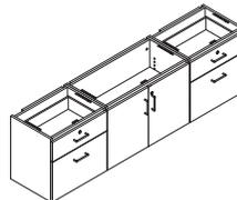
**Bolts** are used to align adjacent cabinets in a multi-unit configuration. The bolts can be removed and reinstalled if a different multi-unit configuration is desired. *Tip: Side of cabinet will be defaced by bolts. Exposed bolt holes will require field fix.*
