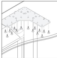
**Worksurfaces** are secured to standard mounting plate for support.
