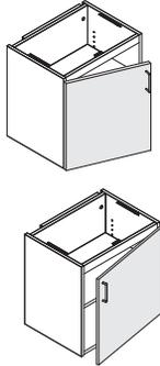
**Single-door cabinets** are hinged on the left or right side. A left-hand unit has the hinge on the left side of the door. A right-hand unit has the hinge on the right side of the door.
