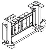
**Technology stretcher** includes CPU straps that allow up to two desk top CPUs or two thin client PCs. ▶ See *Technology Stretcher Computer Capacities*, page 192.
