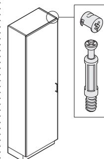
**Cam-lock assembly hardware** is used.
