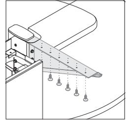
**Worksurfaces** are secured to standard cantilevers for support. Transaction cantilevers are available to support transaction depth worksurfaces and are specified as an option to the base unit.
