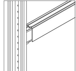
**Convey rails** attach to the structural beam by screwing through the skins. The V.I.A. spacer is required to fill the gap between the skin and the beam. Spacers are not visible once the skin is in place. Spacers span the width of the structural beam.
