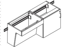
**Base cabinets** attach to a rail system utilizing a bracket connection. The rail aids in alignment to adjacent cabinets. The rail must be ordered separate from the cabinet. ▶ See page 168 for rails.
