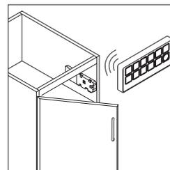
**Electronic locks** are optional and field installed. Lock receivers are installed on drawers and doors and are wirelessly controlled by a transmitter. *Tip: Transmitters are ordered separately.* ▶ See page 174 for electronic locks.
