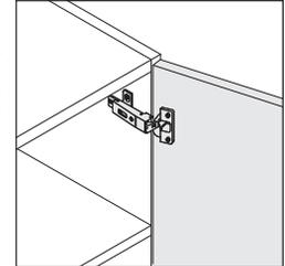
**Euro hinge** is standard on cabinet door and allows the door to open a full 110°.
