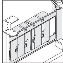
**Open back of technology stretcher** allows power and data access into the technology stretcher from wall.
