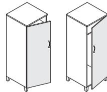
**Single-door cabinets** are hinged on the left or right side. A left-hand unit has the hinge on the left side of the door. A right-hand unit has the hinge on the right side of the door.
