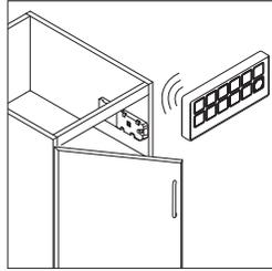
**Electronic locks** are optional and field installed. Lock receivers can be installed on drawers and doors and are wirelessly controlled by a transmitter. *Tip: Transmitters are ordered separately.*
