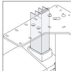
**Vertical cable manager** attaches from stretcher and opens up to work surface.
