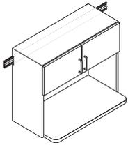
**Upper microwave cabinets** attach to a rail system utilizing a bracket connection. The rail aids in alignment to adjacent cabinets. The rail must be ordered separate from the cabinet.
