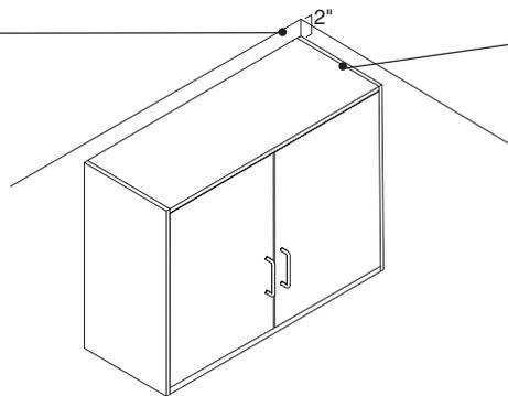
**Convey ceiling fillers** are scribe-to-fit components which are designed to fill these gaps.
