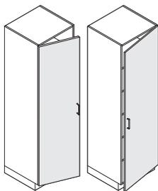
**Single-door cabinets** are hinged on the left or right side. A left-hand unit has the hinge on the left side of the door. A right-hand unit has the hinge on the right side of the door.
