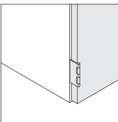
**Five-knuckle hinge** is optional and allows the door to open 270° or 180° if connected to adjacent cabinet.
