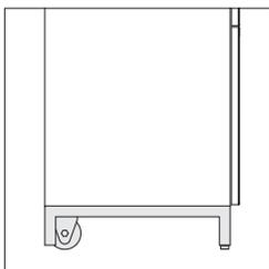
**Rear rollers and front glides** are optional to assist in moving the table. Rear rollers are non-directional and are placed adjacent to the rear legs.
