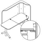
Desk mounted wraps give a 1" gap from the back of the worksurface to the front of the screen.
