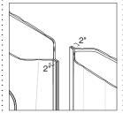
**Aligning** of boundary units to reduce gaps where sound can travel allows for optimal acoustic performance.
