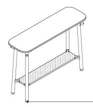
**Glides** provide 1" of leveling and are used for installation on uneven floors.
