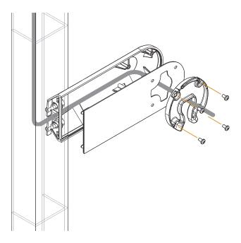
10 Route the PoE network cable though the mounting puck and insert it into the RoomWizard. The RoomWizard will power on once an active network cable is connected to the unit.
