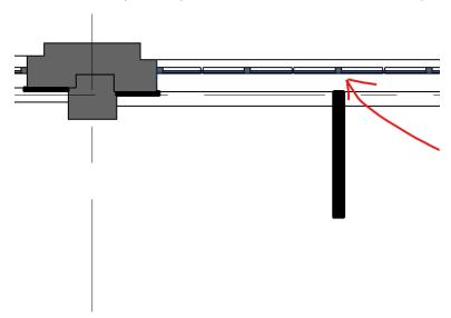
A: Yes, this could be accomplished; however, we wouldn't recommend. For walls that engage with the perimeter, we recommend that students consider walls along the column lines. Walls at the window mullions would be more involved to detail and execute than walls at the columns; however, are permitted if this is what best meets the student's design intent/needs for their project.
