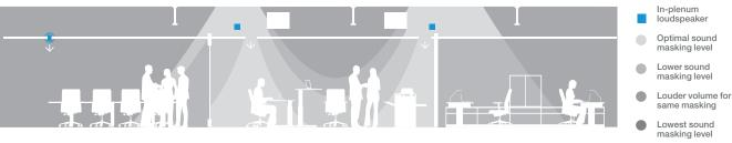
In-plenum systems fall short. Plenum-based sound masking systems project sound upward with use speakers above the ceiling. Beams, HVAC components and other obstructions above the ceiling affect how sound filters into the workspace. Sound is inconsistent and unpredictable, and requires tedious tuning to achieve even coverage.
