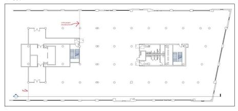
A: The red dashed lines on the plan are the project boundary lines for the space NEXT has rented. Students must provide demising walls in these locations and the space to the left of these boundaries are considered out of scope (NIC). Therefore, the main entrance into the NEXT space is plan south of the elevator lobby.
