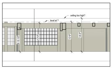
A: The actual slab to slab dimension is 12'- 0" and this is what should be used for the competition.
