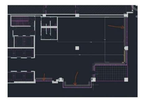
**A:** The items in question are vents that are part of the building HVAC system. These vents are located on the floor and cannot be removed or covered with any material. They can be seen in the photos of the unfinished space that are linked in the Resources section of the NEXT website. They are along the windows.
