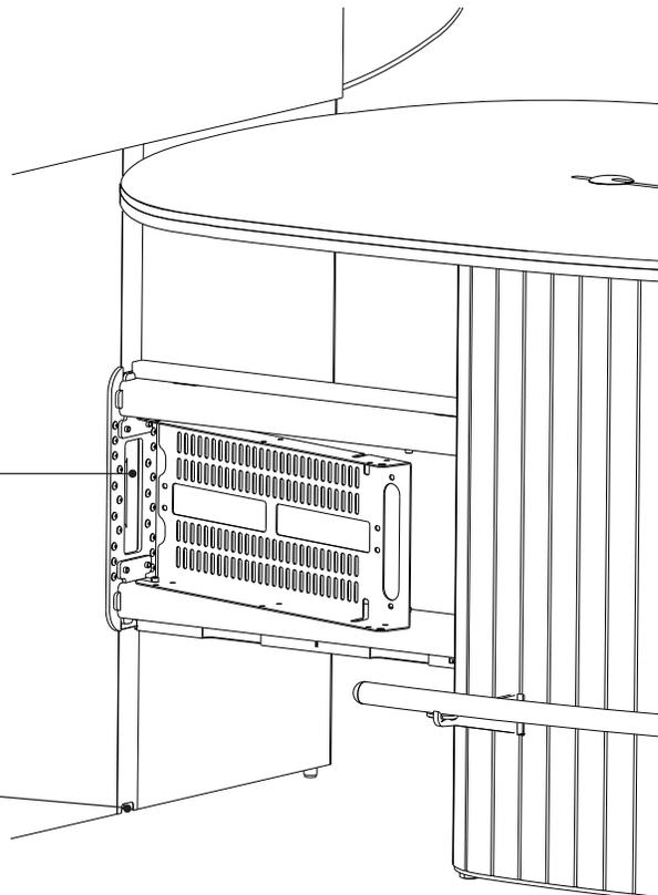
**Tech panel** houses the cables from the channel cover and routes them to the base of the table. The door does not require tools to take off, simply lift and remove to reveal the tech tray to neatly arrange the wires.
