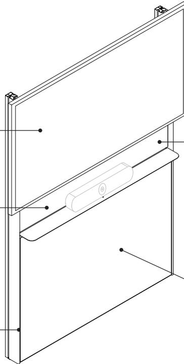
**Camera shelf** is included for foot mounting cameras and sound bars allowing for a simple and flexible installation within the space. The camera shelf is paint matched to the specified frame paint color.
