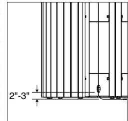
**The cable pod** used as the counterweight (the pod below the worksurface) should be placed at least 2 inches above where the cable rests above the floor. For optimal use, each cable should be fitted with two pods - one above the worksurface and one below to keep connections in place and provide a counterweight for stability.
