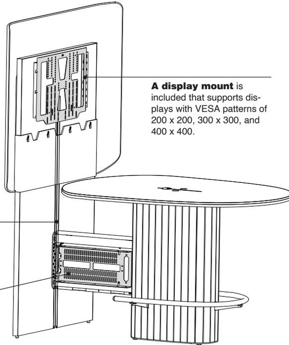
**A display mount** is included that supports displays with VESA patterns of 200 x 200, 300 x 300, and 400 x 400.
