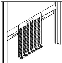
**Tech panel** utilized for mounting AV technology and power components is accessible behind the access door and can slide along a horizontal support to accommodate existing power and data outlet locations at the wall.
