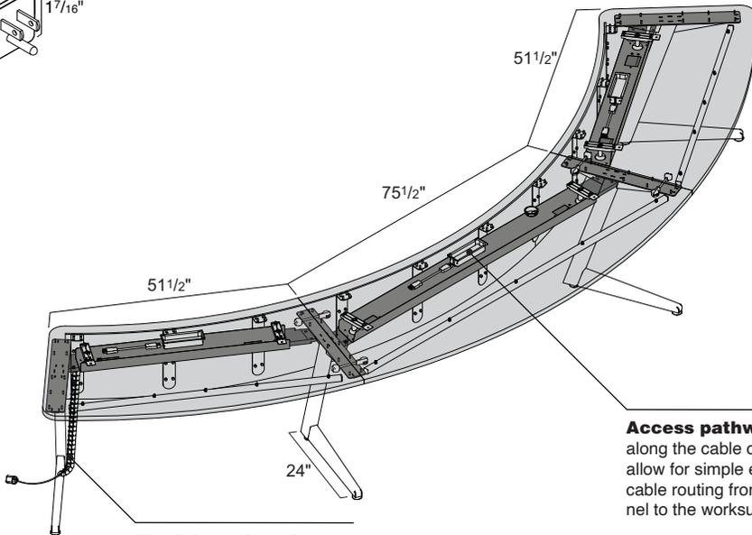
**Flexible options for covering and routing all power and data cables** are available up the table legs.
