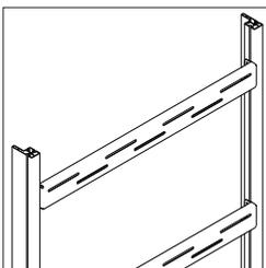
**Horizontal wall attachment** includes seven different slot openings that span the entire cross section to ensure that the desired attachment point at the wall can be utilized.
