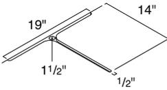
**Aperture cutout** is 19" x 14" x 1/2". There is a 1 1/2" opening in the center of the aperture.
