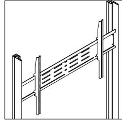
**VESA display mount** is included and supports display configurations with VESA hole patterns up to 1100W x 600H.
