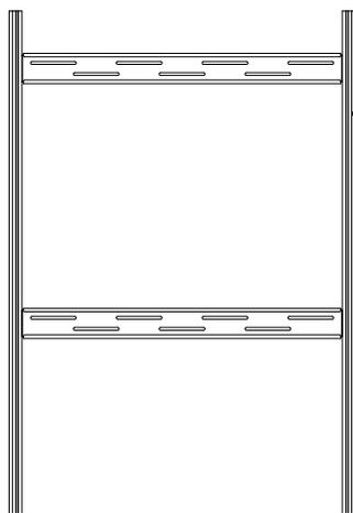
**Ocular frame** must be fastened to the wall by two different connection points along each of the two horizontal attachment beams.
