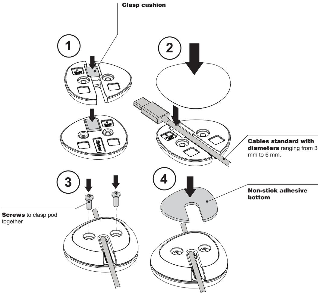
**Cable pods** are clasped together via two screws. A non-slip adhesive bottom is provided for each pod and is easily applied over the screws once the desired clasp tension is achieved.
