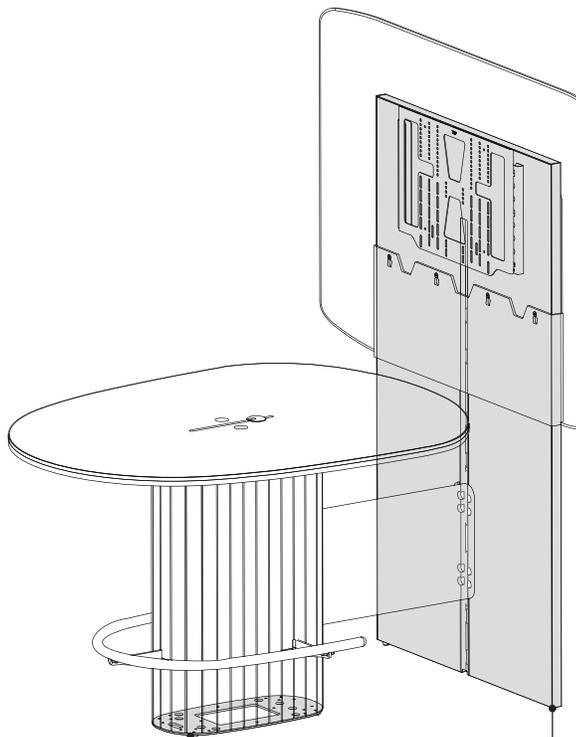
**The tower base** has an access port at the bottom for an alternative route for power and data cables to make their way into the structure.
