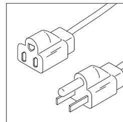
**Standard NEMA 5-15 three-prong plug** connects to building power.
