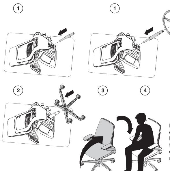
Note: Sit in chair to securely lock components together and complete assembly
