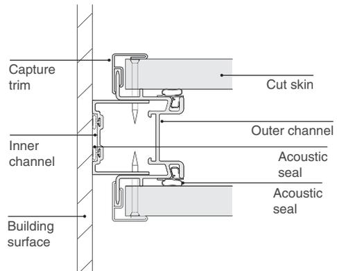
**Cutable ends** can be used at straight cuts to adapt to site conditions or dimensional changes.
