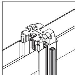
**Frame couplers**, ordered separately, join panels together. They prevent light and sound leaks and run from the top of the glass frame to the floor, overlapping the floor track.
