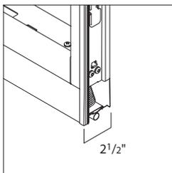
**Structural frames** are approximately  $2\frac{1}{2}$ " thick to accommodate an overall wall thickness of 4".
