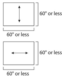
**When the skin size is 60" or less in width and height**, the grain pattern can be specified to run vertically or horizontally.
