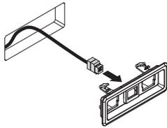
**A modular communication faceplate** can be used to create voice and data terminations using a design that is consistent with modular power receptacles.
