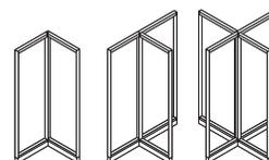
**Adapters** connect panels in L-, T-, and X-configurations without adding extra creep to panel dimension.
