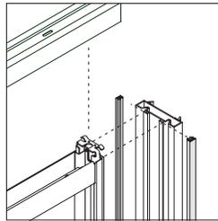
**Adjacent panels** connect to a mini end in the same way all panels connect. Frame couplers on both sides of the panel form a continuous link to the mini end by engaging the verticals of the mini end and the adjacent panel.
