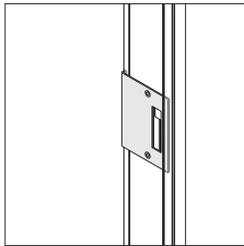
**When specifying single door frames for use with mortise locks,** the strike plate can be specified in either of two configurations. Strike plate type 1 is compatible with the standard Everwall lock, as well as Sargent, Corbin, Russwin, and Yale locks. Strike plate type 2 is compatible with mortise locks manufactured by Schlage and Lawrence. Strike plates are included as part of the assembly hardware kit.
