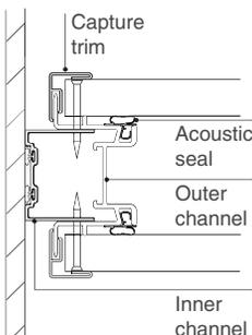
**Inner channel** can be specified in a different color than capture trim.
