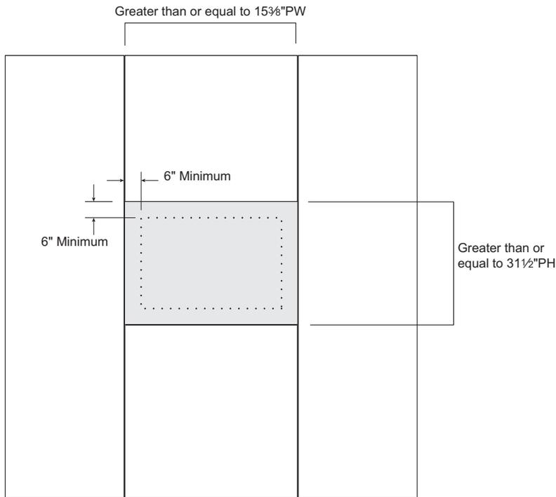
**If skin planning height** is greater than or equal to 31½" and skin planning width is greater than or equal to 15¾", surface mounting of up to 20 pounds is allowed. The item being mounted must project 4" or less from the surface of the skin. The mounting points of the item being hung must be at least 6" from the edges of the skin.
