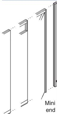
**All panel types and door frames** can connect to a mini end.
