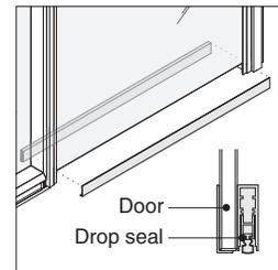
**To enhance acoustical performance,** an optional drop seal can be specified at the bottom of the door. The drop seal automatically deploys to block the gap under the door when the door is closed and retracts when the door is open.
