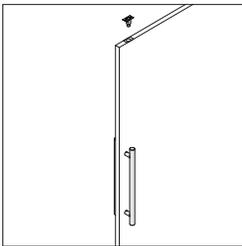
**When specifying a solid door with push/pull or ladder pull,** specify with either a roller latch or surface-mounted closer.
