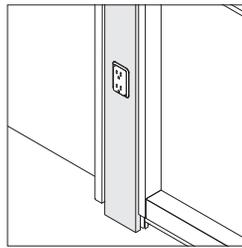
**Utility panels** are used to house electrical devices adjacent to glass panels and door frames, or when skin cut-outs are not desired.
