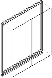
**Everwall frame and glass kits** are assembled in the field. Butt joints must be sealed with glazing tape.
