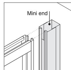
**Mini end** connects a panel or panel run to a perpendicular building wall.
