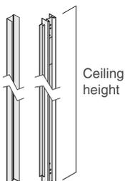
**When intended for use with a single vertical cut**, the inner and outer channel are ordered in lengths that correspond to ceiling height.
