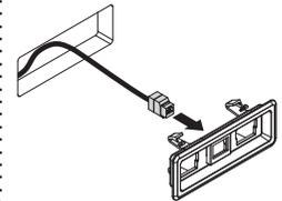
**A modular communication faceplate** can be used to create voice and data terminations using a design that is consistent with modular power receptacles.
