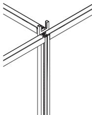
**T-adapters**, can present a cleaner visual than T-posts by presenting a single reveal and ceiling track continuity.
