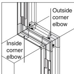
**Cutable end assemblies** can be combined with corner angles and elbows (inside and outside corner) to allow the installer to trim around unique end configurations.
