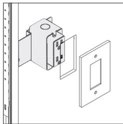
Conventional communication faceplates can be used with an electrical box, which is held in place with electrical mounting brackets.
