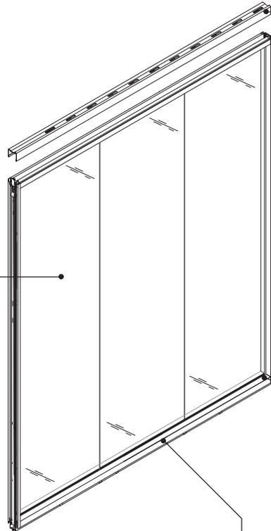
**Ceiling track** secures the top of the Everwall to the suspended ceiling grid. Allows plus/minus 1/2" of adjustment.
