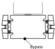
**The planning width for a bypass assembly is 6".**
