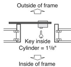
**When ordering cylinders from other suppliers for use with the Everwall slider lever locksets**, cylinders must be specified with a Schlage L cam configuration. When keyway and cylinder are oriented to the outside of the door frame, specify a 2" cylinder with a 7/16" trim ring. When keyway and cylinder are oriented to the inside of the door frame, specify a 1 1/8" cylinder with a 9/16" trim ring.
