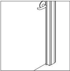
**Mini ends** always go to the floor and ceiling and are field-cut to the proper height.
