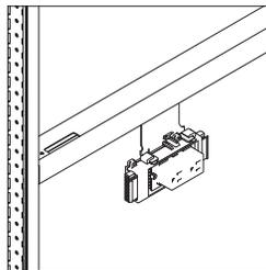
**Modular power blocks** are held in place with mounting brackets, which are fastened to structural frame components.
