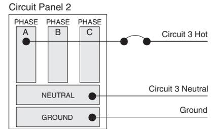
**In the three-circuit, separate neutral schematic,** circuits 1 and 2 are distributed from two different phases from the first circuit panel. Each circuit is supported with its own neutral and a common ground. Circuit 3 is distributed from the second circuit panel and is supported by its own neutral and ground.
