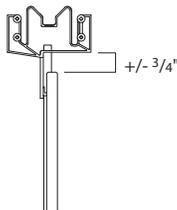
**The visible margin between the top of the door leaf and door frame** can vary by plus/minus 3/4" to accommodate floor variation.
