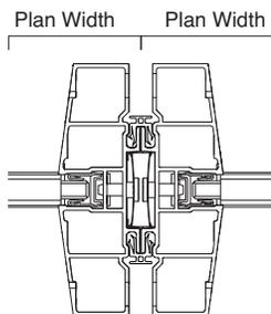
**Plan width of panel** is measured to center of joint between two panels.
