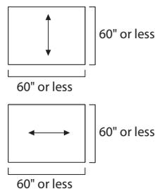
**When the skin size is 60" or less in width and height**, the fabric warp direction can be specified to run vertically or horizontally.
