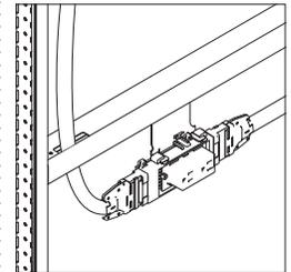
**Each power block** can receive a single harness at either end.
