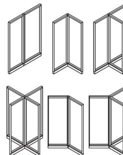
**Posts** join panels in in-line, L-, T-, X-, V-, and Y-configurations without blocking access to integral slotted verticals.
