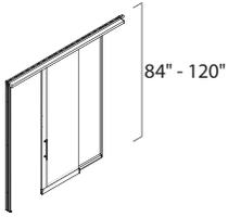
**Door frames** are available in full height configurations. Height range: 84"–120" ceiling height.
