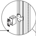
**Electrical mounting brackets** support hard-wired or modular power.
