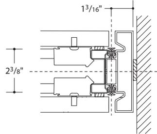
**Finished-end adapter** caps the exposed vertical edge of the last panel in a run. Surface of the adapter is painted or anodized aluminum. Finished-end adapter adds approximately 1 1/16" to the length of the wall.
