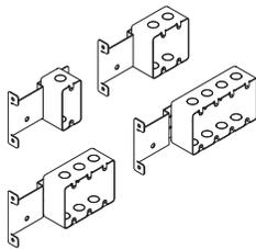
**Mounting brackets** can accommodate single gang, two gang, three gang, or four gang junction boxes. Mounting brackets are designed for use with 2 1/2" deep junction boxes as manufactured by Appleton. Single Gang – M1-250 Two Gang – M2-250 Three Gang – M3-250 Four Gang- M4-250 Partition – LVP250 Skins can be factory cut for any of these four sizes.
