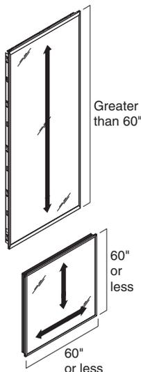
**Certain glass patterns** may have a linear pattern. When one of the glass frame dimensions is greater than 60\", the linear direction will run parallel to the long dimension. When both frame dimensions are less than 60\", the user can specify if the pattern is to run vertically or horizontally.
