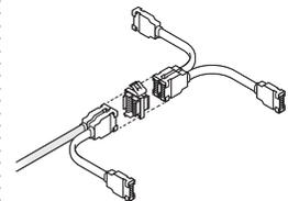
**Harness-to-harness branching connector** link harnesses. This allows multiple harnesses to connect at a single point to allow power networks to branch.
