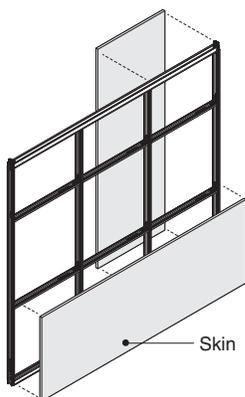
**Skins** can span up to four structural frames, and multiple intermediate horizontals. Different configurations are allowed on opposite sides of the wall.
