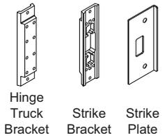
Hinge Truck Bracket Strike Bracket Strike Plate
