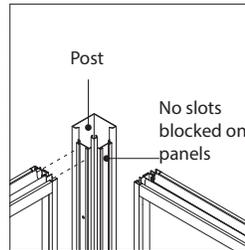
Slotted verticals are accessible when using posts.
