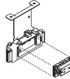
**Receptacles** are ordered separately and field installed in power blocks. Separate duplex receptacles are available to engage each of the different circuits that are possible in the electrical system. Receptacles are coded to indicate which circuit and type of ground they engage.
