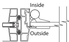
**When specifying doors with etched glass**, the etched surface can be oriented to either face of the door. Specify inside orientation when the polished face is oriented on the same side as the hinge knuckle. Specify outside orientation when polished edge is on the opposing face.
