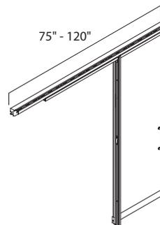
**The slider track** is available in width from 75" to 120", in 1/16" increments.
