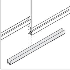
**Floor grippers** can be used to provide additional lateral support at the floor on carpet or hard surfaces, utilizing the simple option specification. They are required when used in active seismic zones as directed by the structural engineer of record, utilizing the seismic option specification.
