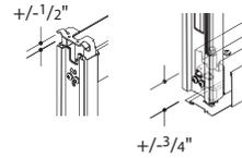
**Ceiling track** allows 1/2" of vertical adjustment to accommodate variations in field conditions. **Floor track** allows 3/4" of vertical adjustment to accommodate variations at base.
