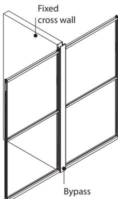
**When applying Everwall glass fronts with conventional fixed cross walls,** it may be desirable to create an interface condition where the Everwall wall conceals the cross wall. The bypass assembly is designed so that it can be installed as a complete assembly and create an uninterrupted visual along a corridor.
