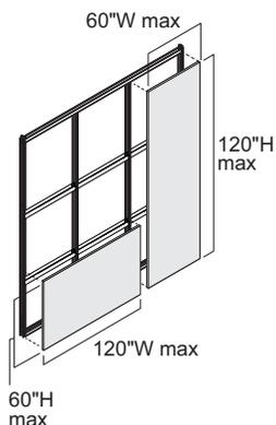
**Steel painted, steel fabric, laminate, laminate markerboard, and fabric skins' maximum planning dimensions** are 120"W by 60"H for landscape planning and 60"W by 120"H for portrait planning. Minimum planning dimensions are 8"W and 12"H.
