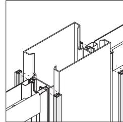
Frame couplers, ordered separately, join posts to panels and door frames. They prevent light and sound leaks and run from the top of the skin or glass frame to the floor, overlapping the floor track.
