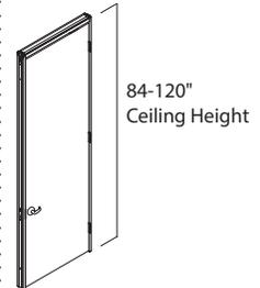
**Door frames** are available in full height configurations. Height range: 84"–120" ceiling height. Heights are specifiable in  $\frac{1}{16}$ " increments. Clear opening height = ceiling height minus  $5\frac{3}{16}$ ".
