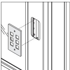
When an electrical box is not desired, communication faceplates can be fastened to the surface of the skin or utility panel.
