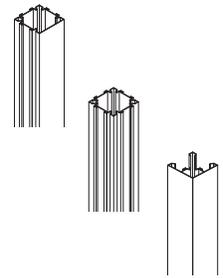
**Posts** span from finished floor to finished ceiling, and are cut to exact length by installer.
