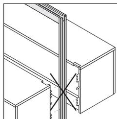
**Panel-supported storage components** cannot be attached to glass wall panels. Use solid wall or Clerestory panels instead.
