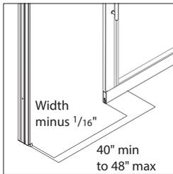
**Door frames** width is parametric and can vary from 40" to 48" planning width in 1/16" increments. Steelcase recommends using a 40" wide door frame to maximize accessibility, maintain visual continuity, and simplify the planning process during reconfigurations.
