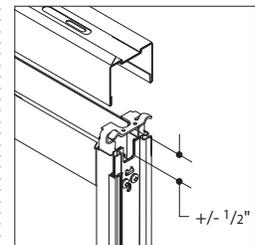
**Ceiling track** comes in 120" and 144" lengths; can be field cut on site. Allows plus/minus  $\frac{1}{2}$ " of vertical adjustments to accommodate ceiling variation.
