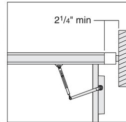
**When mounting a closer on a door and positioning the door at a mini-end,** the door frame must be spaced at least 2 1/4" away from the adjacent surface.
