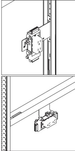
**Electrical devices** are held in place with mounting brackets, which are fastened to vertical structure or intermediate horizontals as part of the installation process.
