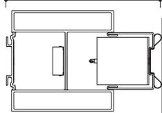
**Two sizes** of mini ends are available. Each telescopes to accommodate a different range of dimensions. For installations that require a dimension smaller than 1 1/2", use a wall start.
