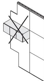
**Cutable ends** do not accommodate hang-on components.
