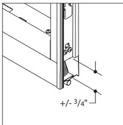
**The floor track** is factory assembled to the structural frame, and serves as the base trim as well. There is plus/minus  $\frac{3}{4}$ " of adjustment to accommodate variations at the floor.
