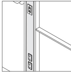
**Utility panels** can include as many as three electrical devices. One of these can be a modular power block. The three cut-outs can be located in one cover, or can be distributed between cover and panel (i.e. two cut-outs in the cover, one cut out in the panel). Utility panel frames and covers can be ordered with factory cut-outs.
