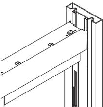
**Finished end** runs from the floor to ceiling, finishing the end of the ceiling track in the same way that the finished end adapter completes the exposed vertical edge of the last panel.
