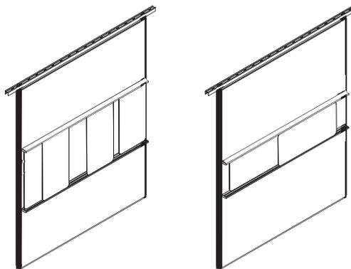
**Flex wall rails** can be installed using brackets engaged into the hanging slots of the Everwall structural frames.
