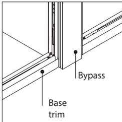
**Bypass assemblies** are designed to be used with base trim along the corridor side of the wall.
