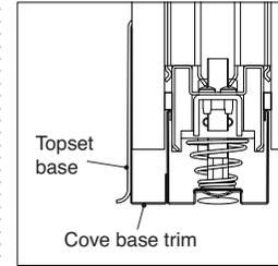
**Additional base trim components** can be specified for use with surface applied cove base. These additional V.I.A. base components are not the finished base material, but serve as surface to receive the adhesive for installation of the topset base material, as manufactured by commercial wall base suppliers. The same base trim components can also be used with applied cove flooring applications.
