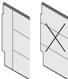
**Cutable end assemblies** do not accommodate intermediate horizontals or segmentation.
