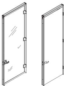
**Door leaves** can be specified as tempered glass with polished edges, or as solid core wood with veneer or painted MDO surfaces.
