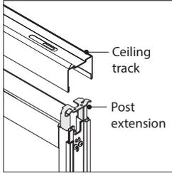
**Structural frames** include an adjustable post extension to ensure connection into the ceiling track.
