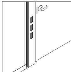
**Utility panels** can be positioned adjacent to door frames to accommodate switches, room schedulers, security control appliances, and other technology devices.
