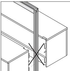
**Panel-supported storage and work surface components** cannot be attached to glass frame kits. Use solid wall or Clerestory panels instead.
