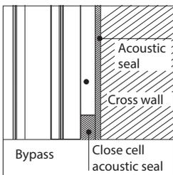
**A close cell acoustic seal** is included to close any gaps between the end of the cross wall and the face of the bypass cover.
