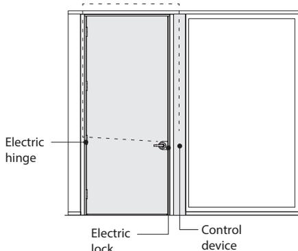
**When door openings** require an electronic security feature, solid doors can be equipped with an electric hinge. The electric hinge includes wire conductors that link an electric lock to the control device (card reader or keypad).
