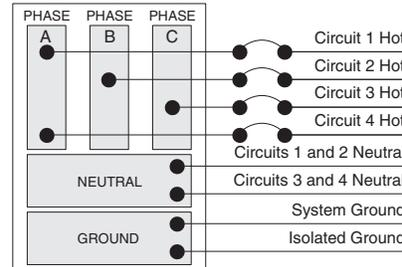
**On a single 3-phase circuit panel,** all four circuits are distributed as shown.
