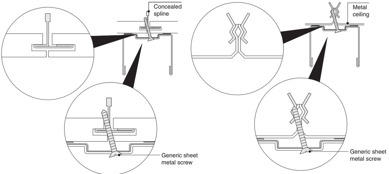
**For these and other types of ceilings, the following fasteners can be sourced locally by the installer:**
