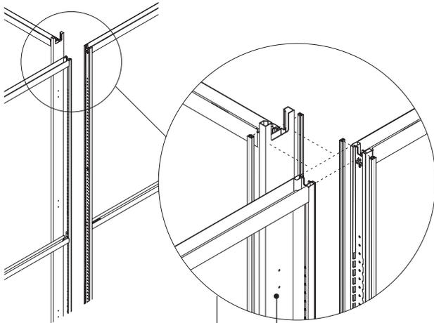
**Surfaces of finished ends and T/X adapters** are painted or anodized aluminum.
