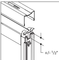
**Ceiling track** comes in 120" and 144" lengths; can be field cut on site. Allows plus/minus  $\frac{1}{2}$ " of floating vertical adjustments to accommodate ceiling variation.
