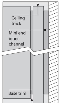
**When making paint color selections**, it is recommended to use the same color for ceiling track and mini end inner channel.
