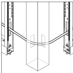
**Infeeds and harnesses** can be fed through posts and utility panels. Horizontal routing holes can be factory-supplied, or cut on-site during installation.
