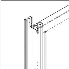
**Frame couplers** ordered separately, join panels and other components to adapters and prevent light and sound leaks. Frame couplers can be cut on site to provide access to the integral slotted verticals so that panel-supported components can be attached. To rearrange panels, frame couplers can be removed and reused.
