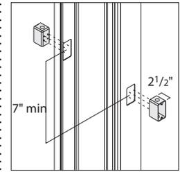
**When hardwired devices using a 2 1/2" deep box** are cut into both sides of the utility panel, they must be offset by a minimum of 7" (center to center).
