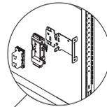
**Electrical mount bracket** at frame vertical.
