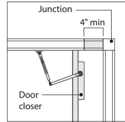
**When mounting a closer on a door, and positioning the door at an inside corner,** the door frame must be spaced at least 4" away from the adjacent surface.
