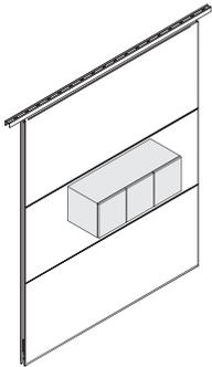
**Storage hang-ons** can be attached to slots in the solid panel and clerestory structural frames with brackets that interface with Elective Elements products. A maximum of two hang-on items can be hung per side of the panel frames.
