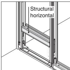
**Structural horizontals that are positioned adjacent to cutable ends** will be modified to ensure that cable cut-outs do not interfere with the bracket connection. These horizontals will receive one cut-out only when 22.61" long or greater. Structural horizontals that are less than 22.61" will not have any cable cut-outs.
