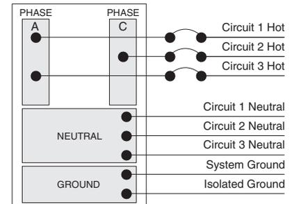
**On a split-phase circuit panel,** three circuits are distributed as shown.
