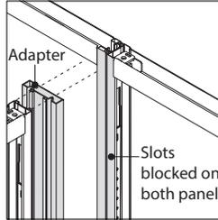
**Blocked slots** occur on the edges of some panels in configurations with adapters. This makes it impractical to attach panel-supported components at these points.
