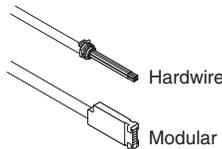
**End of the power infeed** can be hardwire or modular. Hardwire allows the electrician to make a conventional connection to the building's power inside a junction box. Modular allows the infeed to connect to any corresponding modular infeed cover. This is the same modular connector used by Answer, Montage, and Architectural Solutions modular power system.
