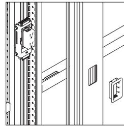
**Electrical devices** are held in place with mounting brackets, which are in turn fastened to utility panel verticals.
