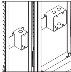
**Junction boxes** are held in place with mounting brackets, which are in turn fastened to structural frame components.
