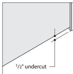
**The door frame assembly** is designed to allow for 1–12" of adjustment at the floor (plus/minus 3/4"), while maintaining a consistent 1/2" undercut.
