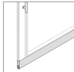
**The polished edge door** includes an adjustable aluminum bottom trim, which can be adjusted during installation to ensure a minimal and consistent clearance at the bottom of the door.
