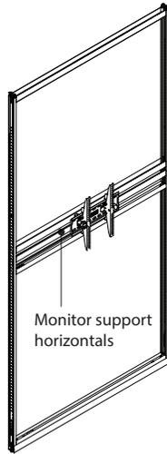
**Monitor support horizontals** come in sets of two and include hardware for anchoring the monitor mount bracket through the skin. Monitor support horizontals are installed on site. Each set has a maximum weight capacity of 200 pounds.
