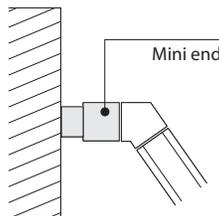
**Mini ends** can be positioned adjacent to an angled post to create an angled wall termination.
