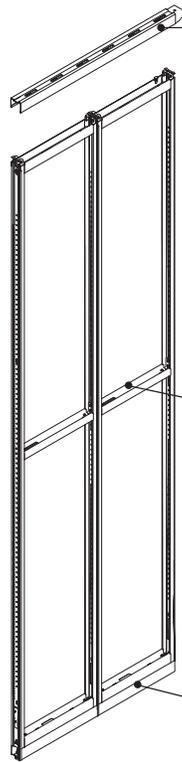
**Ceiling track** secures the top of the Everwall structural frame to the suspended ceiling grid. Allows plus/minus  $\frac{1}{2}$ " of adjustment.
