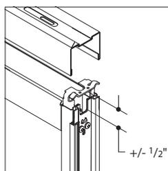
**Ceiling track** allows 1" of vertical adjustment (plus/minus 1/2"), to accommodate ceiling variation.
