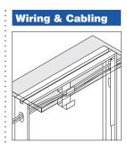
**Cables** can still be routed in the space at the top of a Montage panel when a transaction worksurface is attached in place of a panel top cap.
