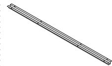
**Reinforcing channels** must be used with tops larger than 54"W for 54"W or more of unsupported kneespace. Any common top used as a table with legs equal to or larger than 30"D x 72"W requires two reinforcing channels.
