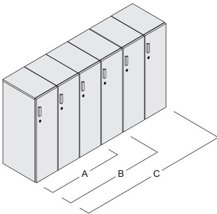
A. Cabinets 70"H or shorter must be attached to two other cabinets, totaling a run of three cabinets.
