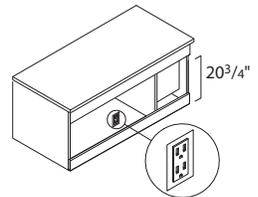
**1/4-height modesty panels** are intended for use up against a wall to provide 20<sup>3</sup>/<sub>4</sub>" of clearance from the floor to the bottom of the modesty panel for all power access, or 13<sup>3</sup>/<sub>4</sub>" of clearance from the top of the bottom stretcher to the bottom of the modesty panel. Top modesty and bottom stretcher are 6<sup>1</sup>/<sub>2</sub>" tall. Bottom stretcher is included when 1/4-height modesty is specified.
