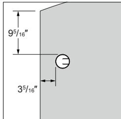
**Corner grommets** are 3<sup>5</sup>/<sub>16</sub>" from the side-edge of the worksurface and 9<sup>5</sup>/<sub>16</sub>" from where the side-edge meets the bow.
