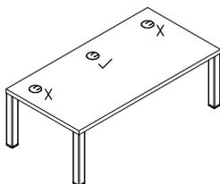
**If creating an application with four legs as supports**, do not specify left or right-hand grommets. Grommet cut out will interfere with leg location.
