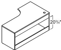
**¼-height modesty panels** are intended for use up against a wall to provide 20¾" of clearance from the floor to the bottom of the modesty panel for all power access, or 13¾" of clearance from the top of the bottom stretcher to the bottom of the modesty panel. Top modesty and bottom stretcher are 6½" tall. Bottom stretcher is included when ¼-height modesty is specified.
