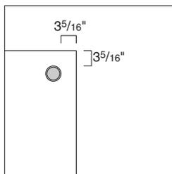
**Corner grommets** are 3<sup>5</sup>/<sub>16</sub>" from the edge of the work surface.
