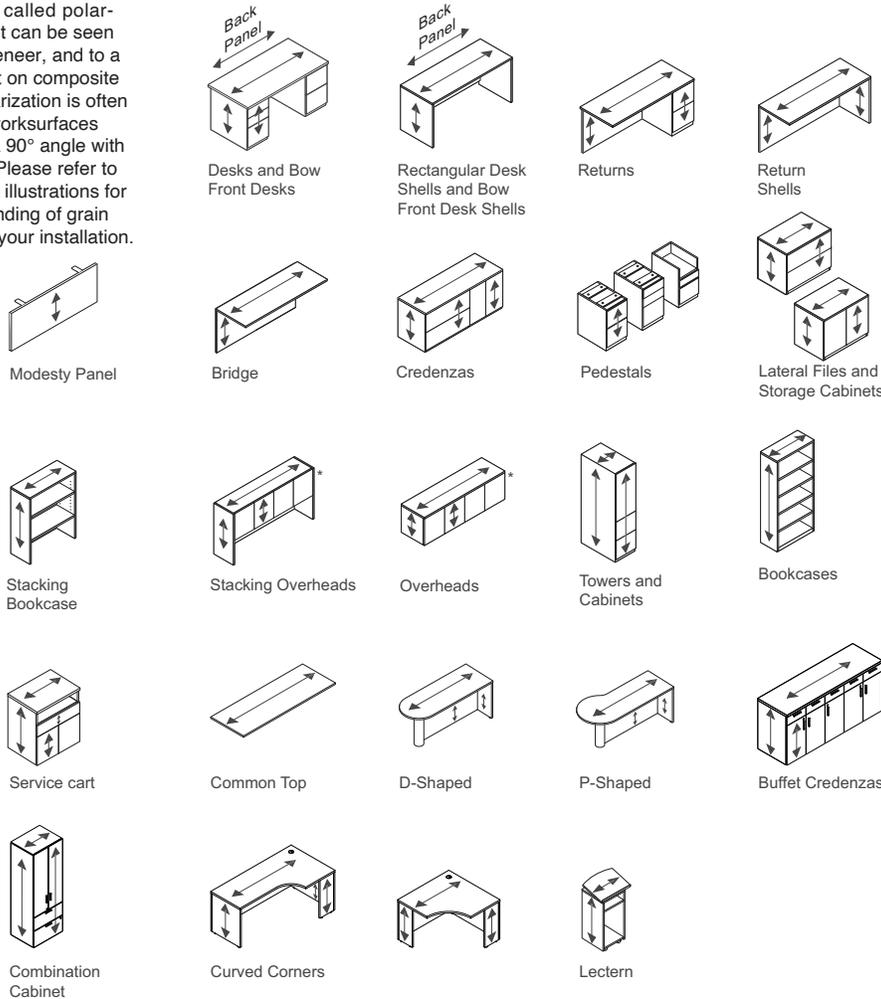
\* 36"W–61½"W overhead back panels have vertical grain direction. 63"W–75"W overhead back panels have horizontal grain direction.
