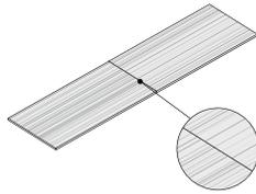
**Low-Pressure Laminate two-piece tops** will not have matching grain patterns.
