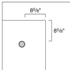
**Corner grommets** are 8 5/8" from the edge of the worksurface.
