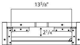
**Interior dimensions of rectangular base** is 13<sup>5</sup>/<sub>8</sub>"W by 2<sup>1</sup>/<sub>4</sub>"D in the center to allow for floor power and data box placement.
