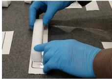
**2.** Firmly press the foam pad onto the hot melt and face shield. Give 10 seconds to cool.
