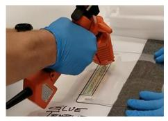
**1.** Apply low temperature hot melt to the face shield with a glue gun.
