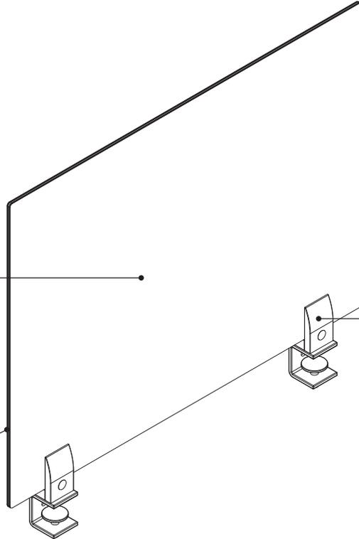
**Boundri screens** are attached with adjustable mounts. 18" and 24" height screens that are available in 24", 36", 48", 60", and 72" widths. The screen and hardware may be used on (nominal) 1/4" to 1 1/4" thick worksurfaces.
