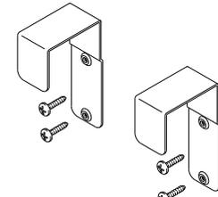
**2" over panel bracket/hook mounting system** allows for Premium Whiteboards to be mounted on Kick and Avenir.
