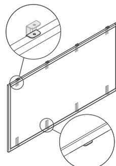
**Wall-anchored mounting system** is standard on 110 and 555 Series.
