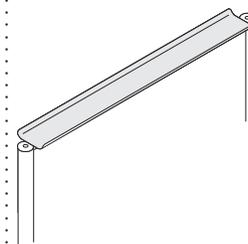
**Marker tray** is available to hold dry erasers and markers. The tray is attached on top of the screen top cap. Marker trays are available in all five screen widths.
