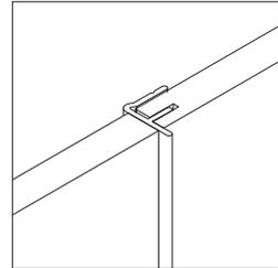
**Accord** features 4 mm protection bumper, material ABS.
