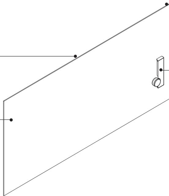
**Edges** are waterjet cut and sealed with high quality paint. Edges show striations.
