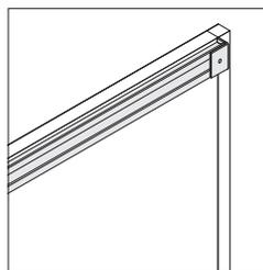
**1" maprail** is of cork construction and allows for versatility with accessories. Maprail is not available on tackboards.
