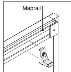
**Roller bracket** holds maps or roll-up projection screens and can be ordered if 1" maprail option is selected. Roller bracket is not available on tackboard.
