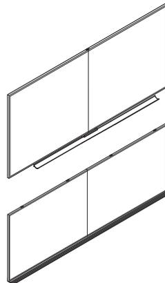
**Spline joints** allow larger format boards to be delivered in two equal pieces and require assembly on-site. There will be a visible seam where the boards and marker trays are joined that will not hinder the performance or writeability of the board in any way. They are available as options with upcharge on Edge, 110, and 555 trim types 120.25" and larger in width.
