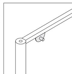
**Flip-chart pegs** are available as an option on the top cap. They are positioned 17 7/8" apart center to center and are available on one side only. Flip-chart peg top cap works in conjunction with marker trays.
