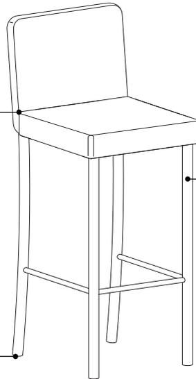
**Legs** feature four tubular steel legs with integrated steel footrests at the front and sides.
