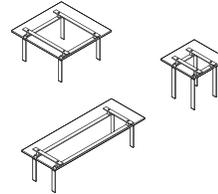
**Occasional tables** are available in three styles: square, rectangle, and side tables. Square tables are available in three sizes: 30"D x 30"W x 15"H, 36"D x 36"W x 15"H, or 48"D x 48"W x 15"H. Rectangle tables are available in two sizes: 20"D x 54"W x 15"H or 30"D x 60"W x 15"H. Side tables are 20"D x 20"W x 20"H. ▶ See *Coalesse Tables, Storage, and Accessories Specification Guide*.
