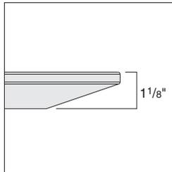
Laminate or wood veneer work surface is standard with a knife edge profile that has the appearance of a 5/8" thick top, which tapers to an overall top thickness of 1 1/8".
