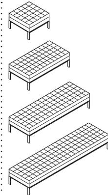
**Benches** are available in 1-, 2-, 3-, or 4-seat. All are 16 1/2"H with four steel legs (1/2" x 1 3/4") with fixed glides. Front and side ganging brackets available.
