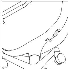
**Seat height** adjusts pneumatically. Lift lever to activate cylinder for desired height. To raise height, slightly stand while lifting lever; to lower, sit while lifting lever and weight pressure will adjust seat height. Range of adjustability is 3 1/2" with a maximum height of 19 3/4".
