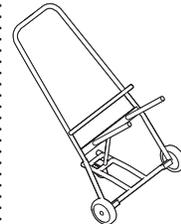
**The Enea Iottus dolly** can be used for storage or easy transport. Chairs stack to six high on the dolly.
