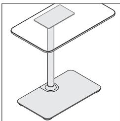
The personal table has a rectangular metal base with the column centered at the back of the base. The 1<sup>1</sup>/<sub>4</sub>" column includes a flat plate at the top that attaches to the underside of the top. The base plate dimension is 10<sup>3</sup>/<sub>4</sub>"D x 15<sup>3</sup>/<sub>4</sub>"W x <sup>3</sup>/<sub>8</sub>"H.
