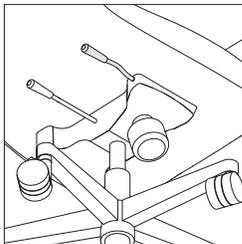
**Upright back lock** allows users to lock the backrest in a full, upright position. To unlock for free tilting, push handle back towards seat.
