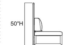
**Two screen heights** are available, 26¾"H for the low-back screen and 50"H for the high-back screen. Seat back cushions extend above the low-back screen, therefore, the overall height of low-back units is 32¾"H. Low-back screens are designed to provide an open environment. High-back screens are designed to provide privacy.
