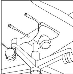
**Seat height** adjusts pneumatically. Lift lever to activate cylinder for desired height. To raise height, stand slightly while lifting lever; to lower, sit while lifting lever and weight pressure will lower seat height. Range of adjustability is 4<sup>1</sup>/<sub>2</sub>" with a maximum seat height of 20<sup>1</sup>/<sub>2</sub>".
