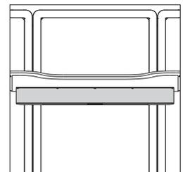
Cable management tray neatly conceals below surface cords to the underside of the work surface.
