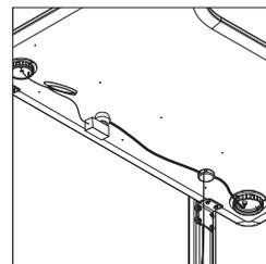
Power package is available when light grommet is specified. Power package includes power module with a below work surface convenience outlet to power the available on-surface light and retain a single power cord out. Specifiable on the back right or back left side of the work surface.
