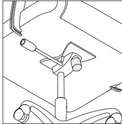
**Tension control knob** allows the user to increase tension (will require more force to tilt chair back), by turning the knob clockwise. For reduced tension and more responsive tilt adjustment, turn knob counter-clockwise.
