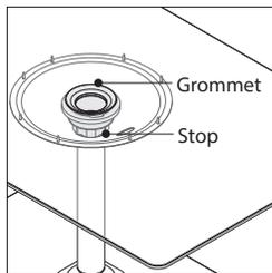
PowerPod grommet and stop is an option on all work and occasional tables. The grommet is located in the center of the table top over the cone/column. The stop attaches to the column to help hold and route cords and cables through the column. The grommet and stop cap are available in black or milk.
