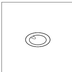
2" light grommet is available to accommodate an on-surface light by routing the on-surface light plug to the below-surface power source. Grommet is specifiable on the left or right side of work surface and is available in three color options.
