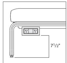
The power and USB power module options are located 7<sup>1</sup>/<sub>2</sub>" from the floor.
