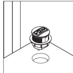
Round power modules are specifiable on the back right or back left side of the work surface. The 3" power module features tamper resistant power simplex, an 8'L power cord with 15-amp plug. Plug includes a built-in circuit breaker measuring 2 1/4"D x 1 1/2"W x 1 1/2"H. Round power module is available in four color options, and three configurations:
