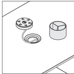
The grommet allows for pass through of cords and cables at the desktop. The grommet is open to allow for the PowerPod to be housed over or stored on the table. The grommet inside dimension is 3 1/2" and outside dimension is 5 1/16".
