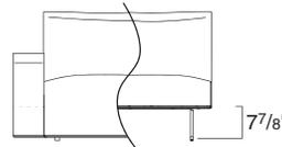
**Additional seam** will be included on arms when fabric is in horizontal/cross direction. The seam location aligns with the height of Sistema lounge with legs for visual connection.
