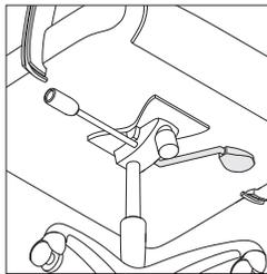
**Knee tilt control (optional)** minimizes the rise of the front of the chair when the chair is in a reclined position, allowing the user's feet to remain on the floor. Push handle up to lock and down to free tilting.
