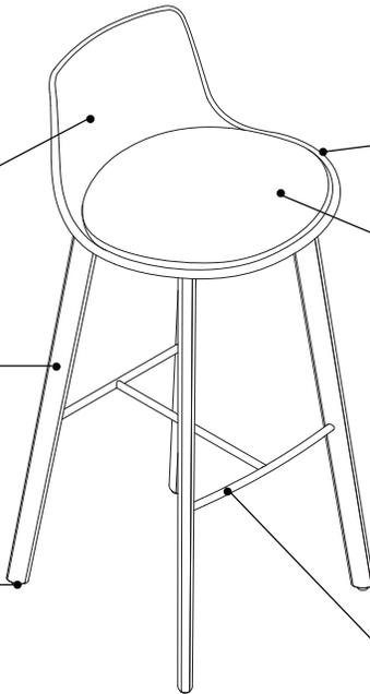
**Casting under the seat** is painted in textured finishes to match polypropylene seat shell.
