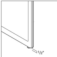
Glides adjust 1/2" for uneven floors. There are two glides per screen. Glides have a metal rounded foot.
