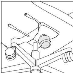
**Back tension control knob** turns clockwise to increase tension and counter-clockwise to decrease tension, allowing free tilt.
