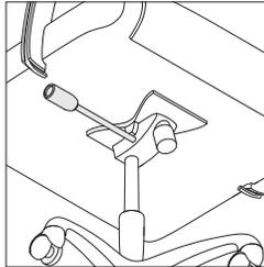
**Seat height** adjusts pneumatically. Lift lever to activate cylinder for desired height. To raise height, slightly stand while lifting lever; to lower, sit while lifting and weight pressure will lower seat height. Range of adjustability is 3" with a maximum seat height of 22".
