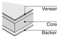
**Wood veneer table tops** are fabricated with Architectural Grade AA hand-selected hardwood veneer, plain sliced, book matched, and bonded to the core with a backing sheet for balance. Coalesse's primary wood finish, Clarity, is a water-borne UV topcoat, which protects the environment while providing exceptional durability and resistance to water and chemical stains. Due to natural variations in wood, finished products may vary from samples in color, texture, and grain.
