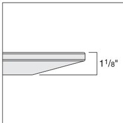
Tables are standard with a knife edge profile, that has the appearance of a <sup>1</sup>/<sub>2</sub>" thick top that tapers to an overall top thickness of 1<sup>1</sup>/<sub>8</sub>".
