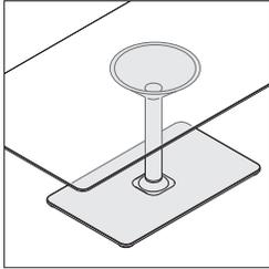
All work and occasional tables have a rectangular metal base with a centered column. The 3" column includes a cone at the top that attaches to the work surface. There are five rectangular base dimensions:
