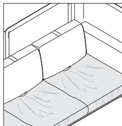
**Comfort wrinkles** are intended to occur over the time to increase the comfort of Lagunitas. Very little maintenance is required to reduce the definition: smooth the cushion fabric with a spreading/wiping motion.
