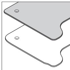
High-Pressure Laminate work surface is standard with a matching or complementing 3 mm flat edge band. Wood veneer tables are standard with a matching wood 3 mm flat edge band. The underside of the table top is finished in black.
