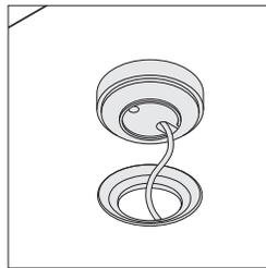
The contour of the PowerPod bottom cradle is designed to work in conjunction with the grommet for a snug fit or can be used independently without a grommet.
