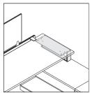
**Intermediate supports** replace the need for other types of worksurface support when used with One-High or 1.5-High Universal storage.
