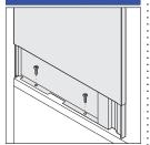
**Hutch end supports** attach to the worksurface using screws that are shipped with the hutch kit.
