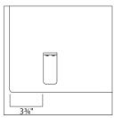
Universal privacy/modesty screen mounts to worksurfaces using simple L-brackets and screws. The brackets are positioned 33/4" in from each side of the
