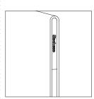
The edge of the screen is comprised of two different materials. The upper segment is merle plastic. The lower portion is PET which can be specified in medium heather grey to provide constrast or dark heather grey for a uniform visual.
