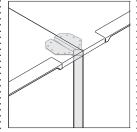
In shared applications, the FrameOne post leg can be angled and positioned at the front edge or for a square orientation it must be inset 1" from the front edge when used with 48"W soft edge worksurfaces.
