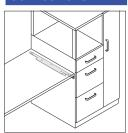
Worksurface to tower connector eliminates the need for other worksurface supports such as legs or end supports next to the tower. ►See page 328
