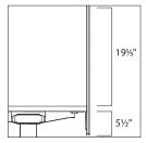
Privacy configuration provides 191/s" of screen above the worksurface and 51/2" of screen below the worksurface. The height is measured from the top of the mounting surface to the top of the screen, and from the bottom of the mounting surface to the bottom of the screen. The top of the screen will align with the bottom of the top trim on a 48"H Answer panel.
