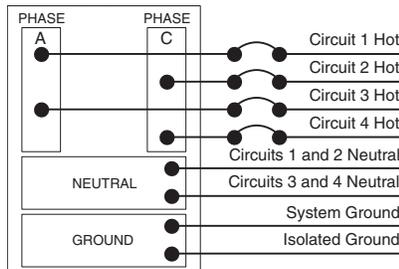
**On a split-phase circuit panel,** all four circuits are distributed as shown.
