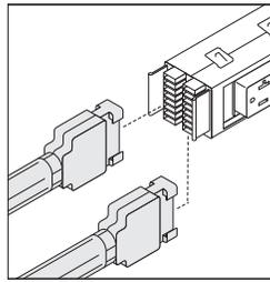
**Harnesses** plug into connection points on the powerkit. Every powerkit has multiple connection points to allow branching of power.
