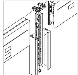
**In-line fence junction** includes junction and in-line fence cover aligner.
