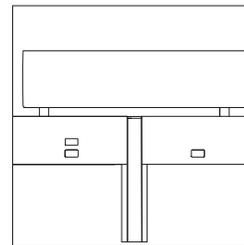
**Universal screen** can span over a junction.
