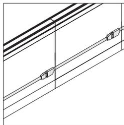
**Pass-through powerkits** extend power between beam segments.
