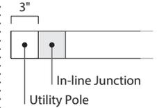
**End-of-run application** uses an in-line junction. Utility pole extends 3" beyond the footprint of the fence.
