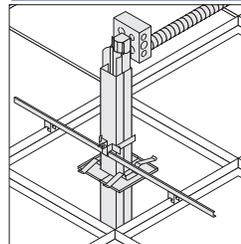
**Ceiling attachment kit** secures the top of the utility pole to the suspended ceiling grid. Hardwired connection to the building's power can be made in the junction box.
