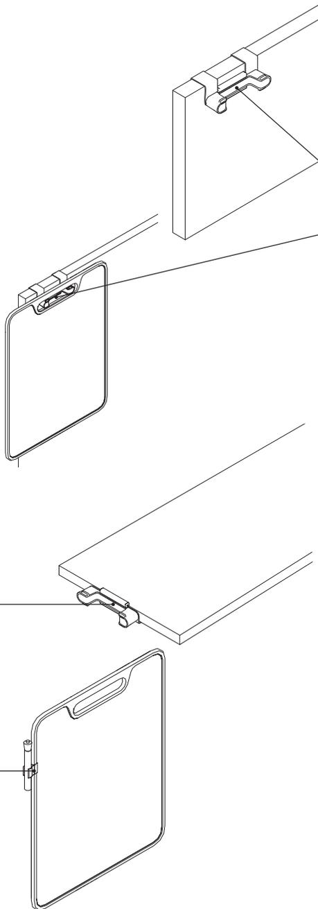
**Verb brackets for boundary screens** are available in double-sided and single-sided configurations.
