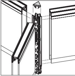
**Y beam junction** includes junction, and Y beam junction cap.
