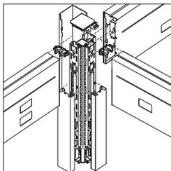
**T fence junction** includes junction, inside corner light seal(s), outside vertical trim, junction cap, and three plastic corner aligners.
