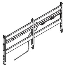
**San Francisco power infeed** can be used if liquid tight conduit is required. Plan to have a long enough infeed to attach to a modular power kit in the beam segment adjacent to the entry panel.
