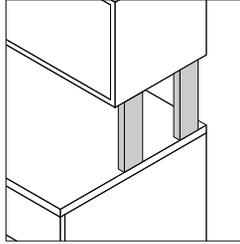
**Single overhead configuration** require two mid-storage supports per end.
