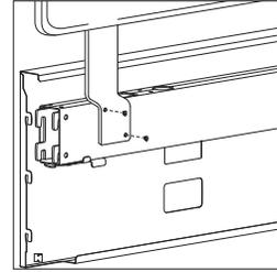
**Sarto screen** can install anywhere along horizontal connecting bar with included self-tapping screws.
