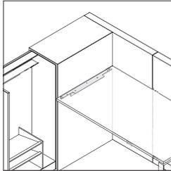
**Worksurface support bracket** can be used to mount a worksurface off one side of the high-density storage eliminating the need for other worksurface supports such as legs or end supports next to the case.
