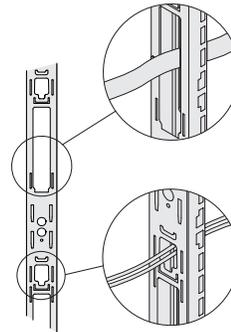
**Horizontal routing of power and cables** can be accommodated through openings in junctions.
