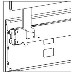
**Universal screen** can install anywhere along horizontal connecting bar with included self-tapping screws.
