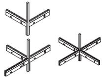
**Utility pole** works with fence. It can be used at an L, T, or X configuration. It cannot be used in an end-of-run, V, Y, or in-line configuration. Utility pole is not shipped with a junction.
