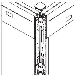
**Block and post construction of corner junctions** allow junction posts to be easily added or removed to configure between L, T, X, V, or Y in an application.
