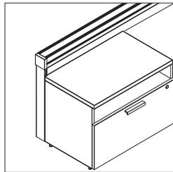
**Storage to beam connector** attaches to One-High, 1.5-High, and Two-High storage to Answer beam to support a beam segment. Connector must attach to a finished back. One-High, 1.5-High, and Two-High storage can not be placed over Answer beam foot.
