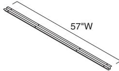
**Worksurface spans greater than 54"** require additional support of a cantilever, pedestal, intermediate support, or leg. Exception: Worksurfaces can span up to 60" in heavy load applications and up to 72" in light load applications if a TS7WKSPPT reinforcing channel is used. Reinforcing channel must be specified separately.
