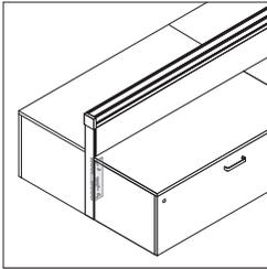
**Low storage-to-beam connector** attaches One-High Currency storage to beams.
