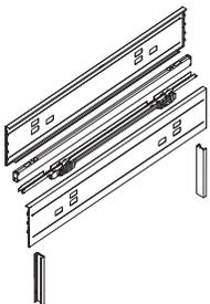
**Answer fence high-capacity horizontal package** includes a horizontal connecting bar, a pair of high-capacity steel covers, a powerkit, and inside vertical trim.
