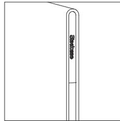
**The edge of the screen** is comprised of two different materials. The upper segment is merle plastic. The lower portion is PET which can be specified in medium heather grey to provide contrast or dark heather grey for a uniform visual.
