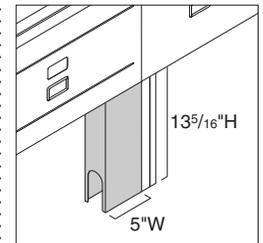
**Infeed cover for high-capacity fence** is 5"D x 13<sup>5</sup>/<sub>16</sub>"H and accommodates up to 70 cables and a multipurpose infeed.
