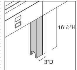
**Infeed cover for standard fence** is 3"D x 16½"H and accommodates up to 24 cables and a multipurpose infeed.
