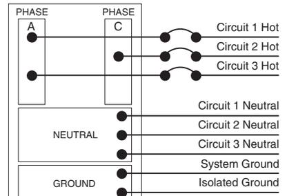
**On a split-phase circuit panel,** three circuits are distributed as shown.
