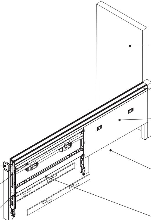
**End-of run cap** matches the beam top cap rail visual profile to provide a seamless finish to the beam.
