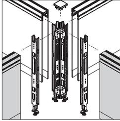
**Posts** can be added or removed from corner junctions to change from one corner configuration to another.
