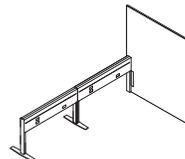
**On boundary screens,** there is a metal cover plate that covers the connection bracket that connects the boundary screen to the end-of-run junction. The cover is located 22" from the bottom of the screen and is 3"W and 14"H.
