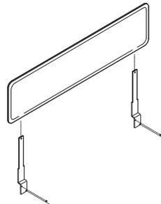
**Sarto screen** slides onto brackets after hard stops are installed on the brackets.
