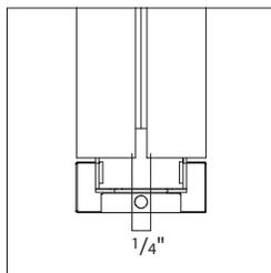
**Steel covers** come together at the top of the fence with a 1/4" gap allowing for use of screens on fence.
