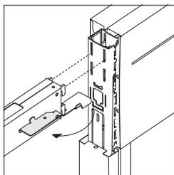
**Quick lock on both ends of the fence horizontal connecting bars** engage the junction in a tight structural connection.
