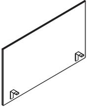
Tip: Universal privacy/modesty screens can be attached to 3/4"-1 1/2" thick worksurface, including height adjustable work-surfaces, universal work-surfaces, and Elective Elements work-surfaces.
