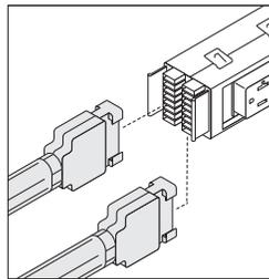
**Multipurpose power infeeds** bring power into the beam and make a modular connection to a powerkit.
