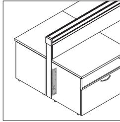
**Medium storage-to-beam connectors** attach 1.5-High and Two-High Currency storage to a beam segment.
