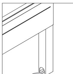
**Infed covers** can be specified for horizontal packages to conceal data cables and power infeed.
