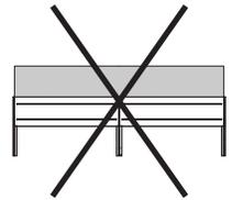
**Frameless glass screens** cannot span over a junction.
