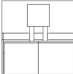
**Overhead storage** supported by mid-storage supports can span two lower storage units.
