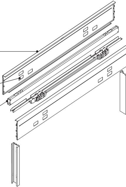
**High-capacity horizontal packages** include taller covers to accommodate additional data cables.
