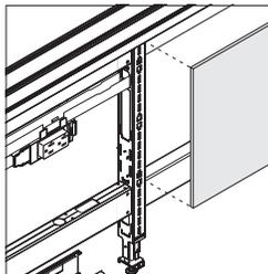
**Skins** extend onto junction and meet skin of adjacent beam segment. The slotted channel of the junction is accessible between these two skins.
