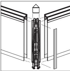
**V beam junction** includes junction, vertical trim, and V beam junction cap.
