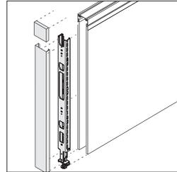
**End-of-run beam junction** includes beam end-of-run junction, beam end-of-run vertical trim, and beam end cap.
