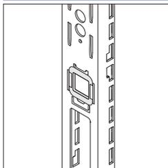
**Grommet for junction** can be added in the field to finish the exposed metal edges of horizontal cable pass-through openings.
