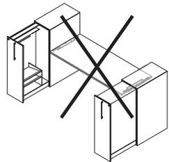
**Worksurface support bracket** can be used to support one side of a worksurface only.
