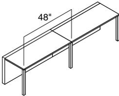
**Reinforcing channel** is not required on worksurfaces with spans less than 54"W.
