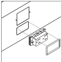
**A receptacle trim ring (TS7RCT)** is required at each power cutout location for modular power configurations and is specified separately.
