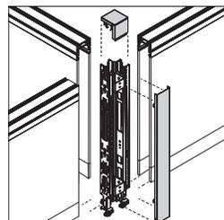
**T beam junction** includes junction, inside corner light seal(s), vertical trim, and T beam junction cap.
