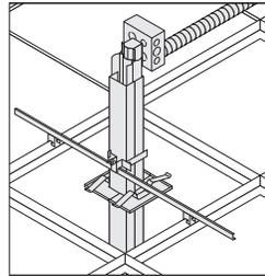
**Ceiling attachment kit** secures the top of the utility pole to the suspended ceiling grid. Hardwired connection to the building's power can be made in the junction box.
