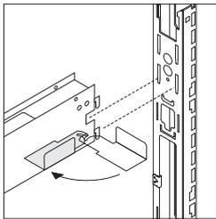
**Quick lock on both ends of the beam's horizontal connecting bars** engage the junction in a tight structural connection.
