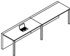
**Reinforcing channel or additional support** is required for worksurfaces with spans greater than 54"W and less than 72"W in light use applications and on worksurfaces with spans greater than 54"W and less than 60"W in heavy load applications.
