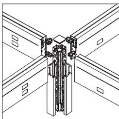
**X fence junction** includes junction, inside corner light seal(s), junction cap, and four plastic corner aligners.
