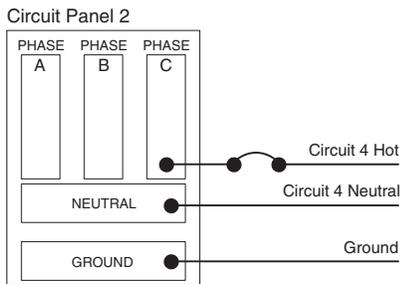
**In the four-circuit 3+1 schematic,** circuits 1, 2, and 3 are distributed from the first circuit panel and are supported with one shared neutral and one shared ground. Circuit 4 is distributed from a second circuit panel and is supported with a separate neutral and ground.
