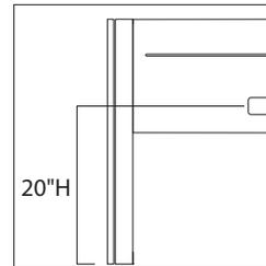
**Power and data** is always expressed at 20"H off the floor to center line of the receptacle with data above the power. The horizontal cover has cutouts to express the receptacle and data cutouts.
