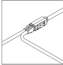
**T-connection** is formed by connecting two harnesses to a power block.
