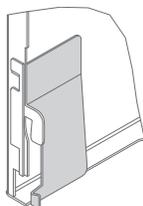
**Covers** include a steel spring clip to lock the cover in place.
