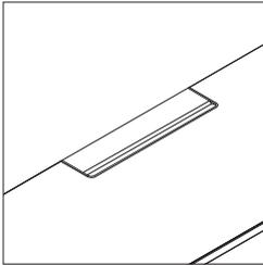
**Power access door** is optional on square edge top for beam and allows access to power receptacles in the beam.
