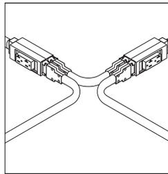
**X-connection** is formed by connecting two harnesses to two successive power blocks.
