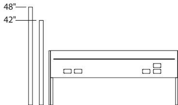
**Fence boundary screens** have modular heights and widths. Parametric widths are allowed from 27"W to 75"W increasing in 1/4" increments.
