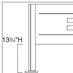
**High-capacity horizontal package** includes vertical trim to create a 13 3/4"H open base.
