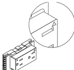
**Orange triangle** indicates to users the receptacles that are connected to isolated grounds.
