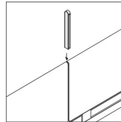
**When fabric screens are placed directly adjacent to each other in-line**, a small aligner can be placed in between the screens at the top to connect them for planar alignment. Aligners are ordered separately in packages of 10.
