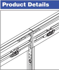
**Power harnesses** are required to connect powerkits between fence sections.
