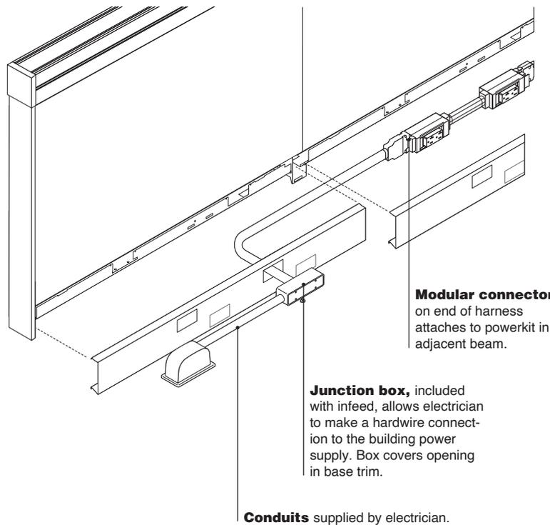
**Order** New York City power infeed of the width that corresponds to the width of the beam it will be installed in. *Tip: Remember that the beam with the New York City power infeed installed cannot accommodate any receptacles in the base because a powerkit cannot be installed. Install a powerkit higher in the beam to accommodate receptacles or use adjacent beam segments to install receptacles.*
