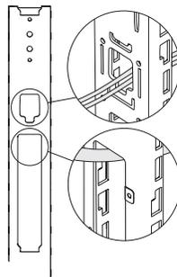
**Answer fence junctions** have the ability to support cabling by routing cable through openings in the junction.
