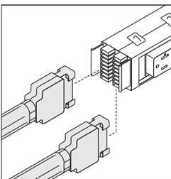
**Multipurpose power infeeds** bring power into the fence and make a modular connection to a powerkit.
