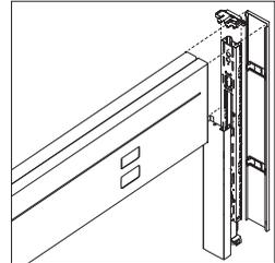
**End-of-run fence junction** includes junction, outside vertical trim, trim aligner, and junction cap. End-of-run trim adds ½" to footprint.
