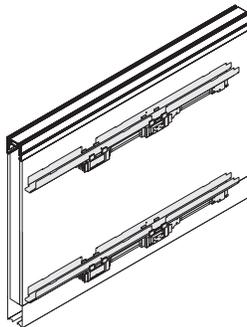
**Powerkits** can be installed in the base, just above the base or 20"H from the floor.
