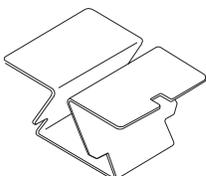
**An in-line fence cover aligner** is included with in-line junctions.
