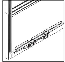
**Power harness** for use with utility pole is available to bring power down from the ceiling and into the beam to make a modular connection to a powerkit.
