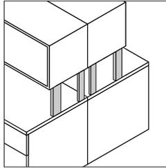
**Overheads in back-to-back configuration** cannot share a center mid-storage support. Two mid-storage supports must be used side by side.
