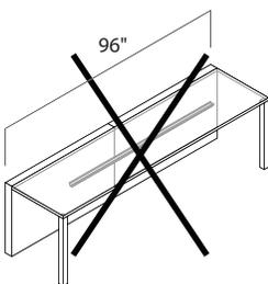
**Worksurface span** cannot be supported solely by a reinforcing channel. Additional to the floor supports are required.
