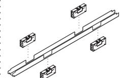
**Junction boxes** are typically mounted below the power tray; however, they can be mounted above when power is routed in a location other than the panel base. A bracket is included for mounting junction boxes above the power tray.
