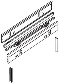
**Answer fence horizontal package** includes a horizontal connecting bar, a pair of steel covers with power and data cutouts, a powerkit, and inside vertical trim.
