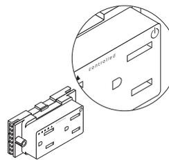
**Controlled receptacle** must be indicated when tying into the building management system. Duplex receptacles have an option for a factory permanent, pad stamp power icon symbol with the word controlled per compliance with the Energy Code.
