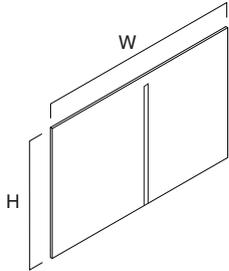
**Beam End-of-Run Straight Boundary Screens—Spanning**
