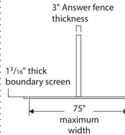
**Spanning fence boundary screens always** extend in equal dimension from the fence to which they attach and include the 3" thickness on the Answer fence. Minimum width for a spanning boundary screen is 51" (48" inside, and 3" for the Answer fence thickness). The maximum width is 75" (72" inside and 3" for Answer fence thickness). *Tip: The above image shows a 75" specified width. The planning width is 72".*
