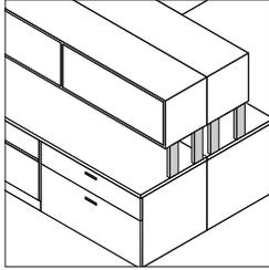
**Mid-storage supports** attach to 1.5-High and Two-High laminate storage or beam-tethered worksurfaces to support the opposite end of stanchion-mounted storage on an Answer beam.
