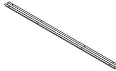
**Worksurface spans greater than 54"** require additional support of a cantilever, pedestal, intermediate support, or leg. Exception: Worksurfaces can span up to 60" in heavy load applications and up to 72" in light load applications if a TS7WKSPT reinforcing channel is used. Reinforcing channel must be specified separately.
