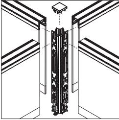
**X beam junction** includes junction, inside corner light seal(s), and X beam junction cap.
