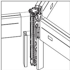
**Y fence junction** includes junction, junction cap, and two plastic top cap aligners.
