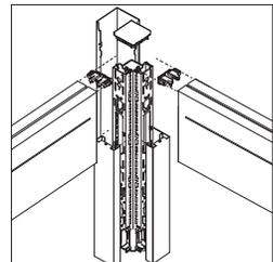
**L fence junction** includes junction, outside vertical trim, inside corner light seal(s), junction cap, and two plastic corner aligners.
