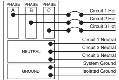
**On a single 3-phase circuit panel,** three circuits are distributed as shown.
