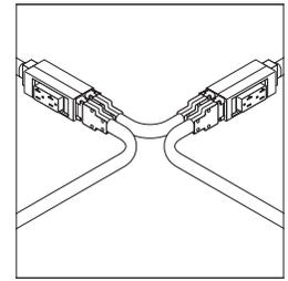
**X-connection** is formed by connecting two harnesses to two successive power blocks.
