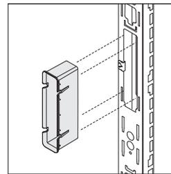
**Junction tall sleeves** can be ordered to cover the exposed metal edges in the large cable routing opening of junctions.
