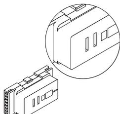
**USB receptacles**, are available in three wiring schematics with multiple line options. USB receptacles offer easy access to two charging ports. Each port provides one ampere of output. USB receptacles conveniently charge a wide range of electronic devices. Some devices may not be compatible.
