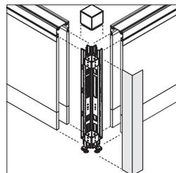
**L beam junction** includes junction, inside corner light seal(s), vertical trim, and L beam junction cap.
