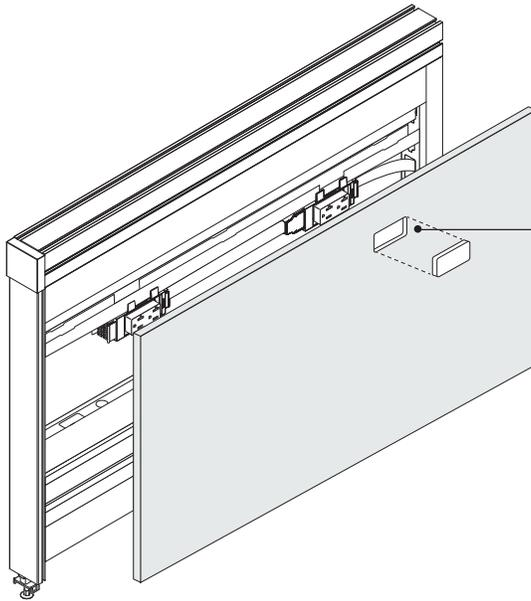
**Power and communication** can be accessed at 20" and just above the base by cutting skin in the field. Templates for cutting both receptacle and communication cutouts are available from Service Parts (T500940SR). Filler to close unwanted cutout in a skin is available from Service Parts (TS7STFSR).
