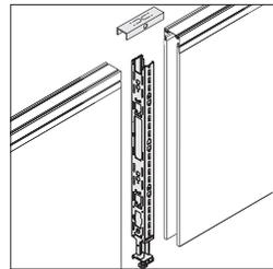
**In-line beam junction** includes beam in-line junction and beam top cap rail aligner.
