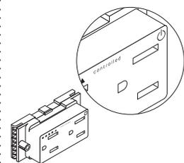
**Controlled receptacle** must be indicated when tying into the building management system. Duplex receptacles have an option for a factory permanent, pad stamp power icon symbol with the word controlled per compliance with the Energy Code.
