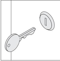
**Locks** are available factory- or field-installed. Factory-installed locks are standard and available keyed random only. Optional field-installed locks are available with consecutive, specific, and random keying options. Master-keyed locks are also available. Field-installed lock cylinders must be specified separately.
