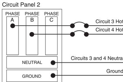
**In the four-circuit 2+2 schematic,** circuits 1 and 2 are distributed from two different phases from the first circuit panel and are supported with one shared neutral and one shared ground. Circuits 3 and 4 are distributed from a second circuit panel and supported by their own shared neutral and ground.
