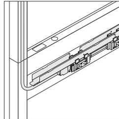
**Power harness** for use with utility pole is available to bring power down from the ceiling and into the fence to make a modular connection to a powerkit.
