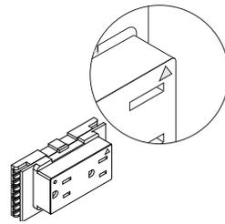
**Orange triangle** indicates to users the receptacles that are connected to isolated grounds.
