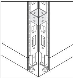
**90° corner and 120° corner junction blocks** can be ordered separately for use in building beam junctions that are not supported by style numbers.
