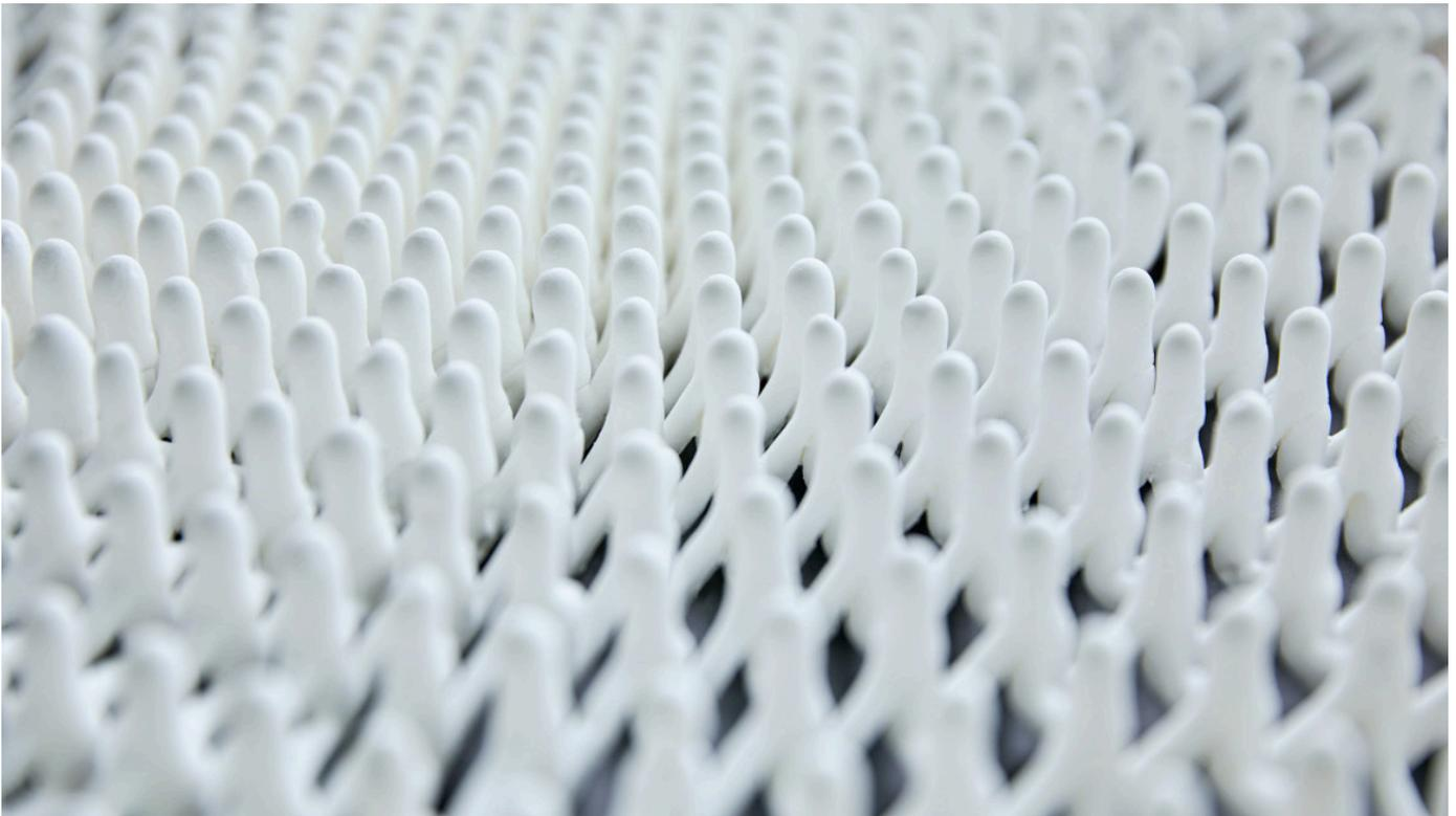
MIT's Self-Assembly Lab, Steelcase and award-winning product designer Christophe Guberan collaborated to create a new 3D printing process unveiled at Milano Design Week. The technology breaks the three constraints of traditional 3D printing by using a rapid liquid printing technique enhancing speed, scale and quality. The partnership between MIT, Steelcase and Guberan explores the future of furniture personalization and the opportunities for customization through innovation.
