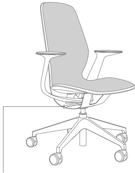
**Seat height** - To raise chair lift body weight up and pull lever up. To lower chair, remain seated and pull lever up. Not available on chairs with swivel auto-return option.
