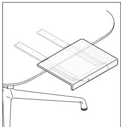
The tablets can be extended 254mm and slide on two runners using a ball-bearing mechanism. They are assembled during on-site installation. The sliding tablets can hold a maximum weight of 10kg. Warning! This product contains grease - risk of stains.
