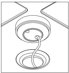
The cable grommet allows cables to pass through the top. The barrier is placed inside the cone and is fixed to the tube, to hold and conceal cables. The cable management fits into the channel inside the base tube to hide the cable routing.
