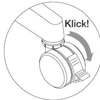
Figure 5-3: Adjusting and locking the casters
