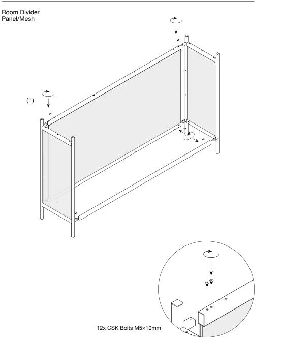
**8.** Attach the brackets to the base of the frame. Ensure they are in the correct position before tightening.
