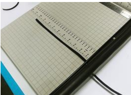
1E. Measure elastic to 25,4 cm (10") and cut. 2 pieces per mask.
