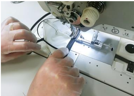
5C. Sew perimeter around entire circumference.
