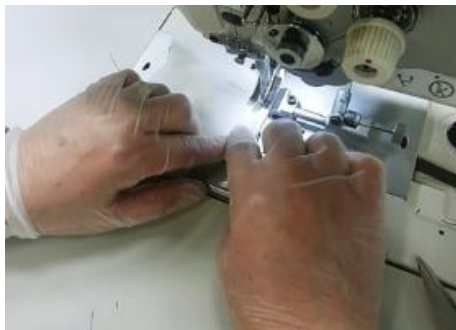
3B. Sew over existing seam as inside out, entire curved seam at 1 cm seam.
