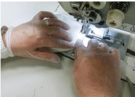
3A. Fold mask inside out and fold at sewn seam.
