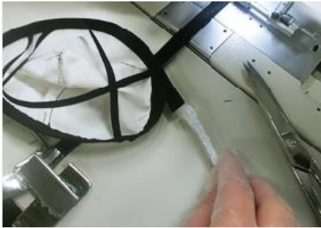
6A. Insert rounded wire end into tunnel.
