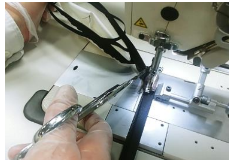
5C. Sew perimeter around entire circumference.
