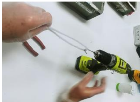
1B. Hold end and run drill 12-15 revolutions until wire end twists.
