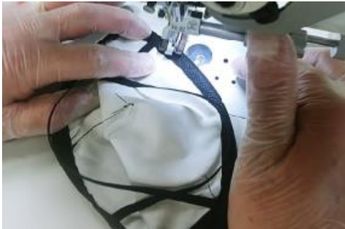
6C. Sew across wire lead end (over the wire) to capture wire.
