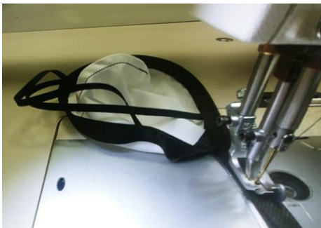
5D. Sew 2,5 cm (1") extended strip off end (at startpoint) and trim.
