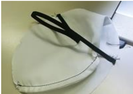
4C. Align and sew strap to opposite upper side notch.
