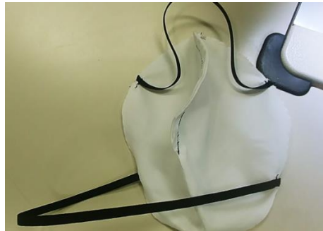
4D. Sew and backtack strap to lower notch edges on both sides. 2 tacks per location.
