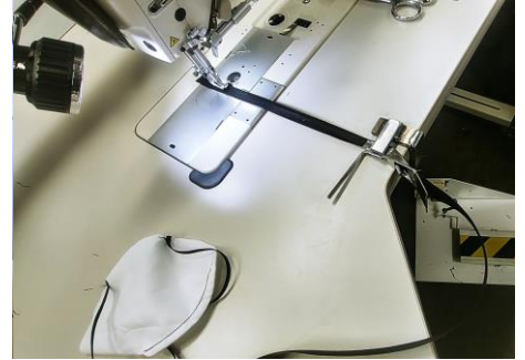
5A. Drawtape fold and drawtape feed.
