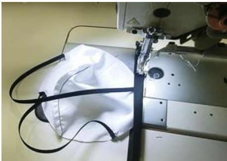
5B. Align fabric edge at strap, fully inserted into drawtape fold.
