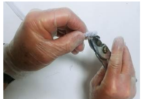
1C. Fold wire end over and crimp tight.
