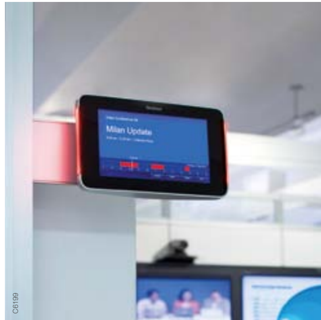
Red light status indicates immediately room unavailability to workers.
