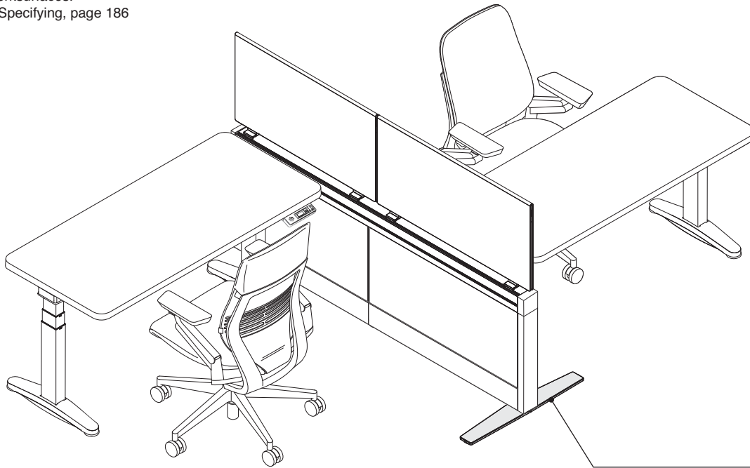
Panel and beam foot
