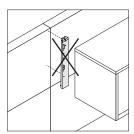
**Horizontal off-module** brackets cannot span a vertical frame rail or joint on enhanced off-module Montage panel only.
