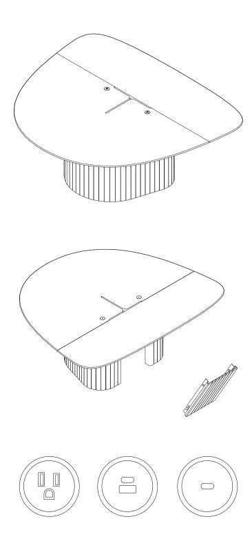
T-shaped aperture cutout is standard with the table and allows for easy, flexible access from above and below the table while also helping future proof for new power and technology systems.
