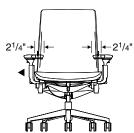
Arm width can be adjusted 21/4" each, 41/2" overall. Grasp arm cap and move in or out.
