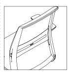
Fabric outer back cover is available on quilted upholstered and upholstered back styles. The fabric back cover conceals the horizontal flexors while keeping the lumbar visible.
