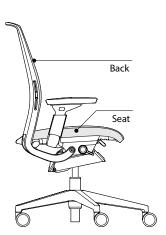
**Seat and back assemblies** can be removed and replaced if damaged.
