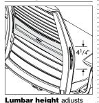
41/4" (6" to 101/4" from seat) by grabbing exposed tabs and sliding the lumbar support up or down. Fixed lumbar height is available as an option on work chairs and stools. The fixed lumbar is positioned 8" from the seat. The adjustment handles are replaced with inserts that fill the lumbar slot in the back frame
