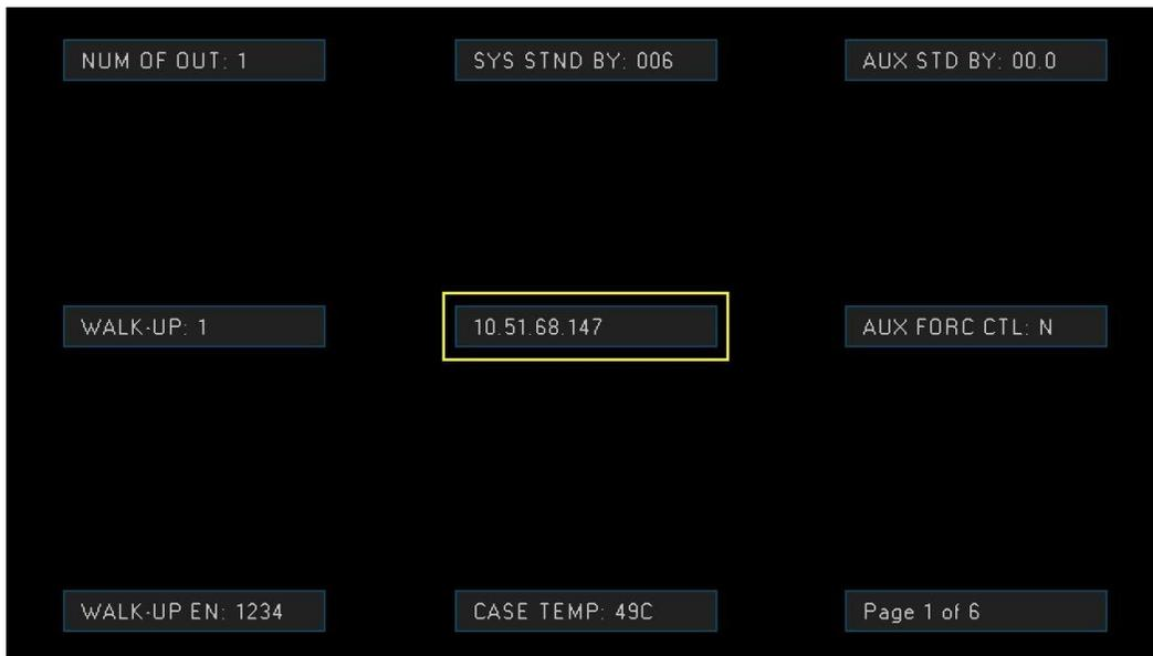
*The switcher's current IP address will be displayed in the center of the screen on page 1 of the OSD.*
