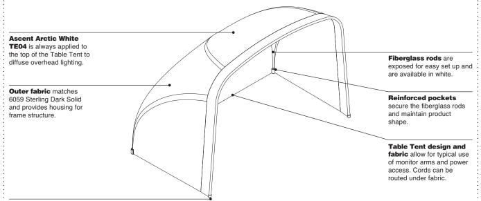
**Rubber stop caps** are included to provide added stability and to protect worksurfaces.
