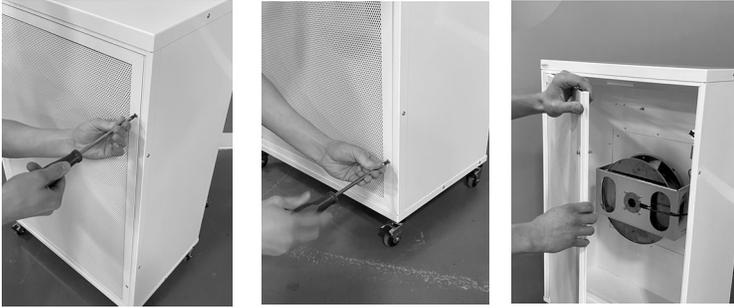
**STEP 1:** Make sure the unit is unplugged and turned off. Remove the two Phillips head screws securing the exhaust grille, these can remain in the grille. Swing the grille open, remove and set aside.
