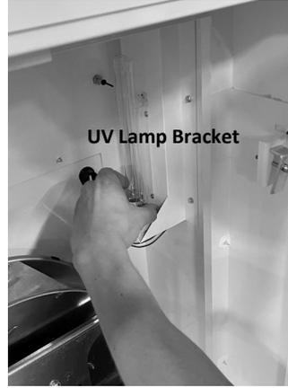
**STEP 1A:** If your unit is equipped with a UV light, install the light by inserting the lamp fixture into the factory installed lamp base and pulling it into place. **Skip to Step 2 if your unit doesn't have a lamp.**
