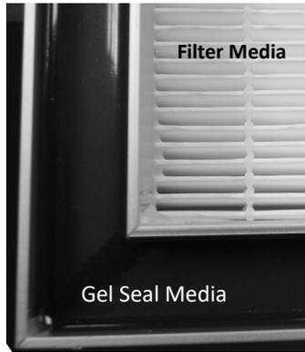
**STEP 4:** The HEPA filter is installed by grasping the sides of the filter frame and placing the filter cell into the housing. The gel, upstream area goes in first and will create the required seal when the filter clamps are fully tightened.
