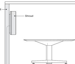
If a table is placed away from the wall, cables can be routed down the column, through the floor, and up the wall to the monitor. When coring the floor 2", conduit is recommended to easily fit the monitor extension cable HD15 connector.
