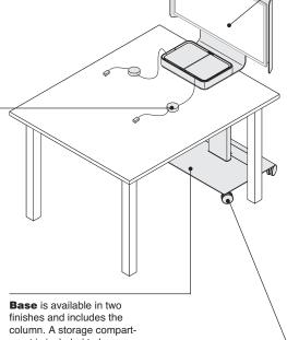
**Casters** allow the unit to move easily. The unit comes with soft locking casters as a standard.
