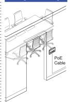
RoomWizard II connects to a network and is powered using Power over Ethernet (PoE). PoE cables run from the PoE switch typically located in the data closet. Industry standards set cable lengths at 100m. Contact your IT department to determine the PoE switch locations.
