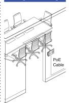
RoomWizard connects to a network and is powered using Power over Ethernet (PoE). PoE cables run from the PoE switch typically located in the data closet. Industry standards set cable lengths at 100m. Contact your IT department to determine the PoE switch locations.
