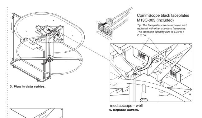
Slotted support structure can fit 5.5"D x 10"W x 1.6"H technology devices or components. Note that this opening exists on both sides of the column.
