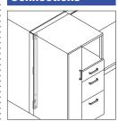
High storage-to-panel connector provides added stability to panels and eliminates the need for return panels.
