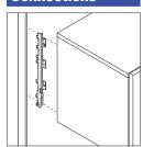
Steel support hooks on end supports insert into the slotted channel of a panel or wall channel and lock into place with a safety catch.
