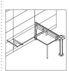
For Montage applications with a combination of panel-mounted and tethered or freestanding worksurfaces with legs, the worksurface(s) supported by legs will not reach the same height as the cantilevered worksurface if panel glides are extended more than ¼". Standard Montage worksurface height is 285%"H when panel glides are at zero. Legs adjust up to 287%"H.
