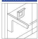
Termination plate is field installed beneath the worksurface in any position needed. Usually, it is located at the back of the worksurface so it doesn't obstruct kneespace.
