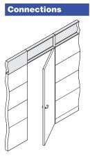
10"H enhanced stacking frames can be used on top of the door frame. The stack-on frame used above the door frame and the door frame should be the same width.
