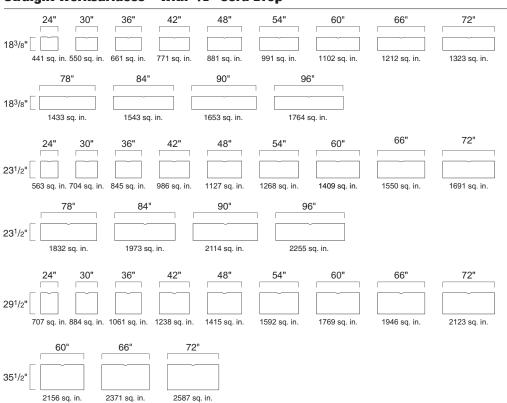
Tip: Worksurfaces greater than 30"D can only be used in freestanding applications.
