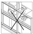
**Glass tiles** cannot be used with worksurfaces because glass prevents the use of cantilevers and worksurface supports.
