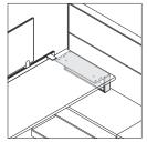
**Intermediate supports** replace the need for other types of worksurface support when used with One-High or 1.5-High Universal storage.
