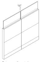
Between adjacent glass, there is a 1/2" gap. Height aligns with a 10"H stacker frame. In-line change-ofheight end trims must be painted version when used beside frameless glass.
