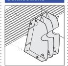
**Slatwall worktools** slide into channels in the slatwall tile. Monitor arms cannot be mounted on a Montage slatwall tile.
