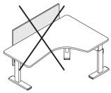
**Boundary screens** are not permitted on height adjustable desks as they do not pass minimum safety requirements which could result in the desk tipping over.
