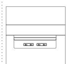
Universal laminate storage with recessed back should be used when storage will be placed in front of a power outlet.
