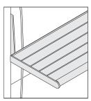
**Gap at back of slim shelf** allows routing of shelf light cord.
