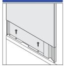
**Hutch end supports** attach to the worksurface using screws that are shipped with the hutch kit.
