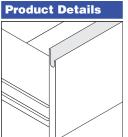
**Flush-front pull** is full width and integral with the drawer. Pull is available on steel drawers only.
