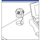
**Power and communication spheres** are field installed. Use a 3"-diameter drill to cut mounting hole at desired location.
