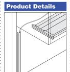
Wire manager is available for use between the bottom of a shelf or overhead storage bin and a worksurface. Wire manager can be cut in the field to suit specific application.
