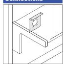
Termination plate is field installed beneath the worksurface in any position needed. Usually, it is located the back of the worksurface so it doesn't obstruct kneespace.
