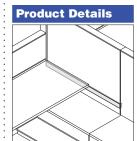
Connects 18"D, 24"D, and 30"D worksurface to wider panels eliminating the need to match panel width to worksurface depth. Replaces side supports, cantilevers, and the need for front edge support with 30"D worksurfaces.
