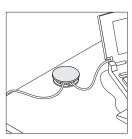
**Lid of port** in up position allows low-profile routing.
