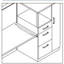
Connects worksurface to tower eliminating the need for other worksurface supports such as legs or end supports next to the tower.
