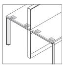
**Half-loop leg** is always panel supporting, however panels cannot exceed 48"H or support overhead storage above.
