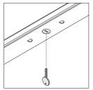
Lock in bin is concealed from view beneath the shelf. Locks are available factory- or field-installed. Factory-installed locks are standard and available keyed random only. Optional field-installed locks are available with consecutive, specific, and random keying options. Master-keyed locks are also available. Field-installed lock cylinders must be specified separately.
