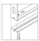
**Heavy steel connectors** bolt to frames to ensure stability. 45"H, 55"H, and 65"H frames can be used by themselves or with one 10"H or 20"H frame stacked on top.
