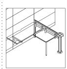
For Montage applications with a combination of panel-mounted and tethered or freestanding worksurfaces with legs, the worksurface(s) supported by legs will not reach the same height as the cantilevered worksurface if panel glides are extended more than ¼". Standard Montage worksurface height is 285%"H when panel glides are at zero. Legs adjust up to 287%"H.
