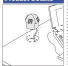
Power and communication spheres are field installed. Use a 3"-diameter drill to cut mounting hole at desired location.
