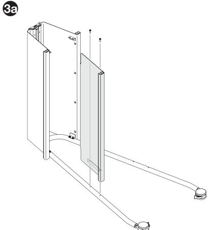
Two (2) M5 X 12mm hex flange head screws Note: Second person required to help steady and keep shelves upright as they are installed.
