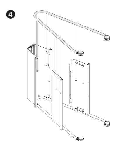
Eight (8) M5 X 12mm, hex flange head screws Note: Second person required to help steady and keep shelves upright as they are installed.
