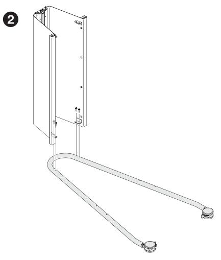
Four (4) M5 X 12mm hex flange head screws Note: Second person required to help steady and keep shelves upright as they are installed.
