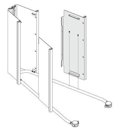
Two (2) M5 X 12mm hex flange head screws Note: Second person required to help steady and keep shelves upright as they are installed.
