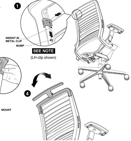
NOTE: Clips may break if coat hanger is removed from chair after successful installation.
