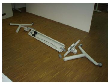
21. After doing this both gearboxes + cantilever are separated from the rest.
