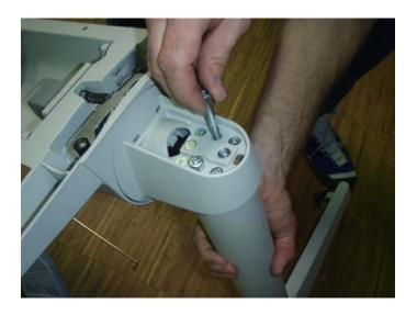
36. Screw both parts together on each side of the frame.
