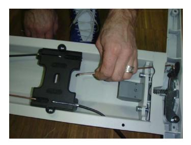
17. Hang out the short primary rod from the deflection unit and from the gearbox.
