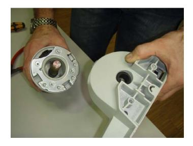
24. Separate the connection flange from the cantilever.
