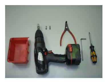
2. Required tools for replacing the gearbox + locking disc inside.
