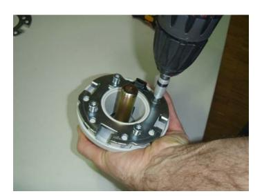
28. Fix the new locking disc with 4 screws.
