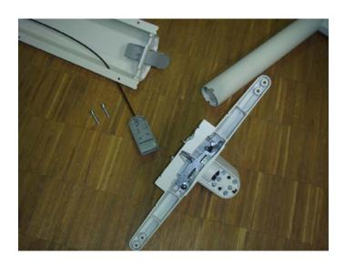
33. Start to connect the gearbox + cantilever with the cable tray again.
