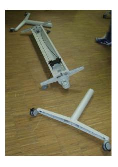
16. Follow the same process for the 2<sup>nd</sup> leg column to have both legs completely separated from the rest.
