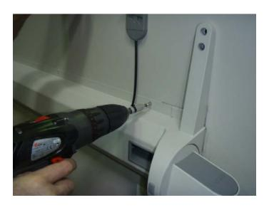
4. The table must be in parking position. Then loosen 8 screws of the cable tray.
