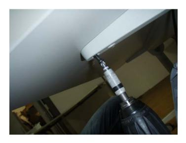
10. Loosen the outer screws of the 4 cantilevers.
