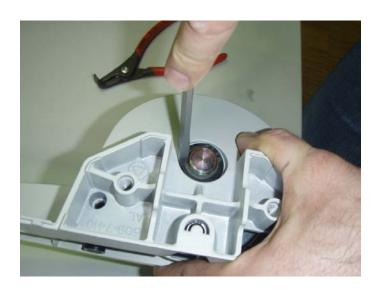
32. Make sure that the locking mechanism is working.
