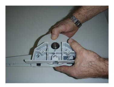
29. Connect the cantilever with the connection flange.
