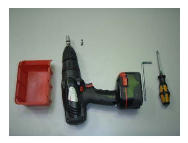
1. Required tools for replacing the gearbox.
