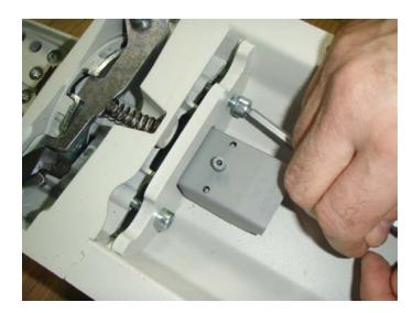
20. Loosen the screws on both ends of the cable tray.
