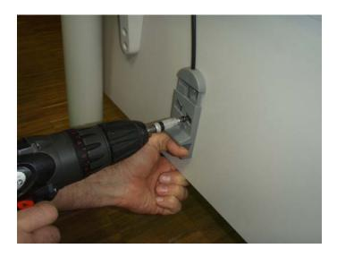
5. Pull the lower handle until the 2 screws can be loosened.
