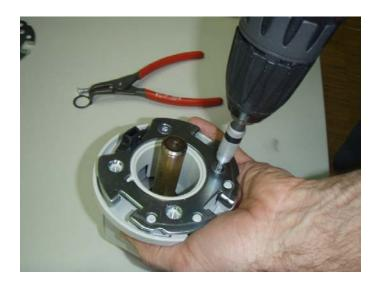
25. Loosen the screws that are fixing the locking disc.
