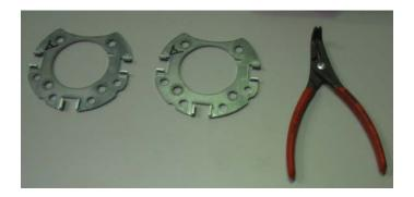
22. For changing the locking disc inside the gearbox a specific pair of pliers is needed.
