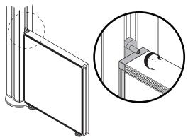
(10) Tighten the set screw until hit the Post to secure the Panel.
