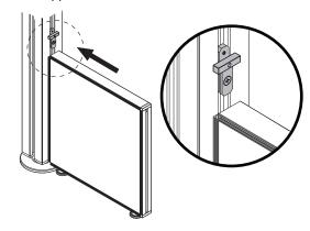
(8) Tighten the screw in order to rotate and lock it to the Post.
