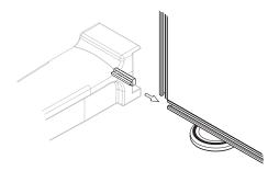
Remove the cap and two screws from stabilizer leg and insert to horizontal slit.
