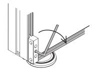
Fix the bracket at the end of slit with slotted set screw.
