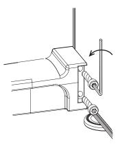
Reset two screws to stabilizer leg from opposite side of corner and fix.
