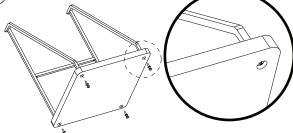
Hook onto the shelf on FE-3 Panel / Screen at desired position.
