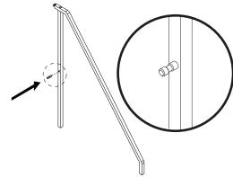
Insert the set screw to the bar and partially tighten it.
